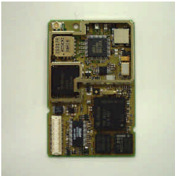
MC46 Module Interior View
