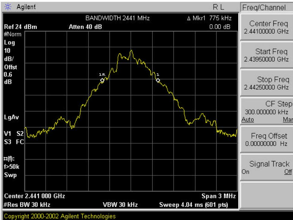
Plot A-2. 20dB Bandwidth Plot – Ch. 45
