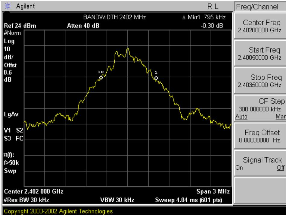
Plot A-1. 20dB Bandwidth Plot – Ch. 01
