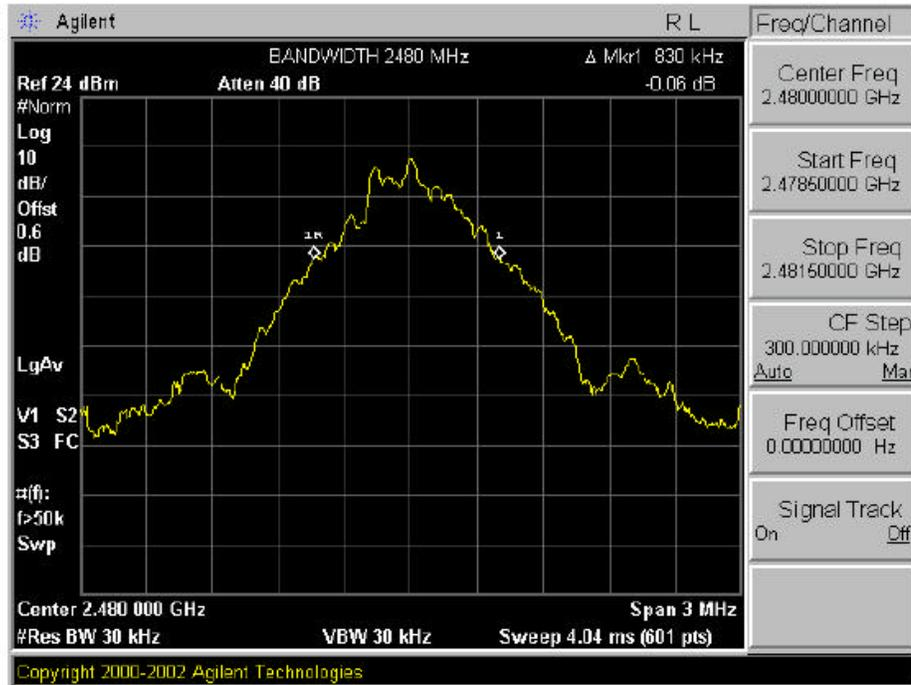
Plot A-3. 20dB Bandwidth Plot – Ch. 79
