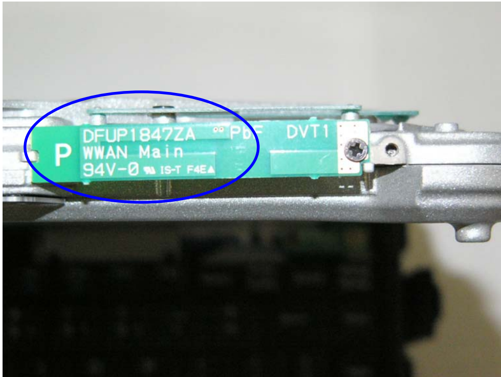
WWAN Main TX/RX Antenna
