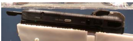
Figure 8-2 CompactFlash radio card in PDA host configuration
