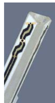
Figure 4-2 Probe Thick Film Technique
