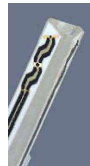
Figure 4-2 Probe Thick Film Technique
