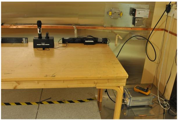
**Power Line Conducted Emissions Test**
