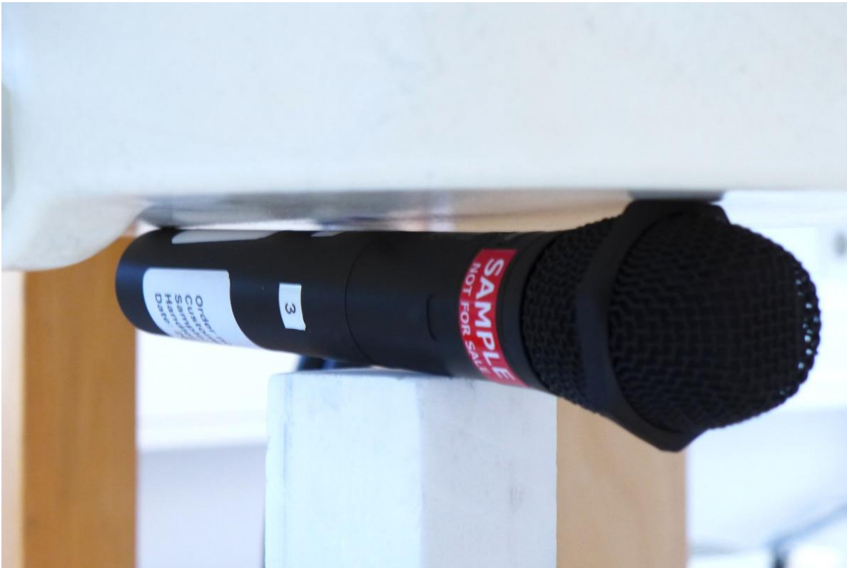
Pic. 4: Test position 2, DUT towards the phantom, 0 mm gap.
