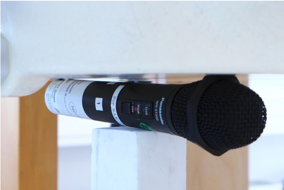
Pic. 6: Test position 4, DUT towards the phantom, 0 mm gap..
