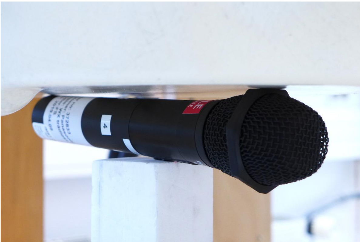
Pic. 5: Test position 3, DUT towards the phantom, 0 mm gap.
