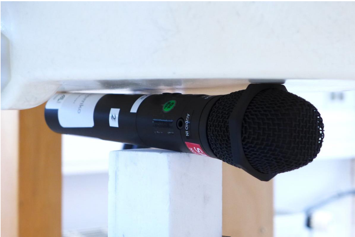
Pic. 3: Test position 1, DUT towards the phantom, 0 mm gap.
