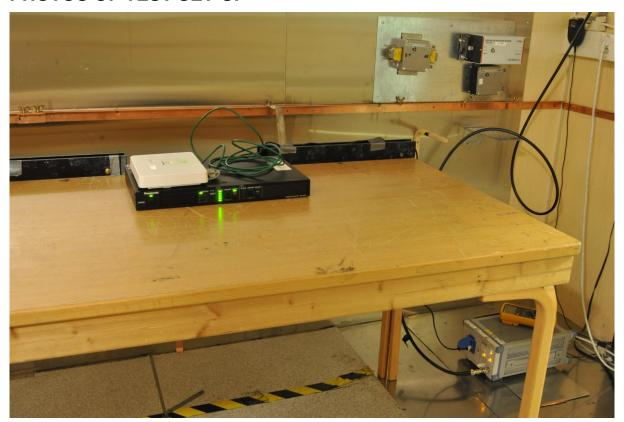
**Power Line Conducted Emissions Test**
