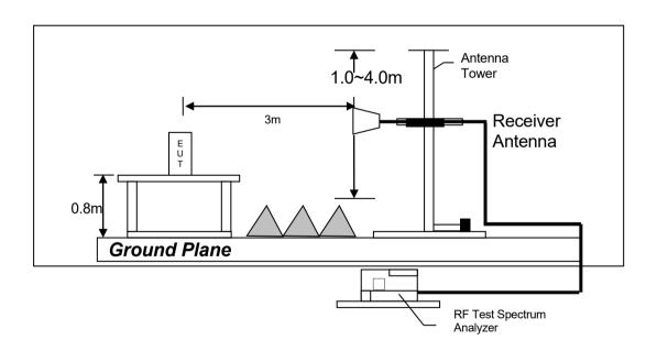
Test setup of radiated emissions above 1GHz
