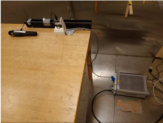
Test set-up for EMC emissions measurements
