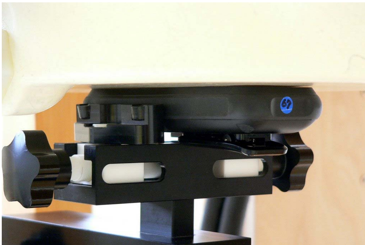
Fig.19: Body worn configuration for KX-UDT131, position 1, display towards the phantom, 0 mm distance.
