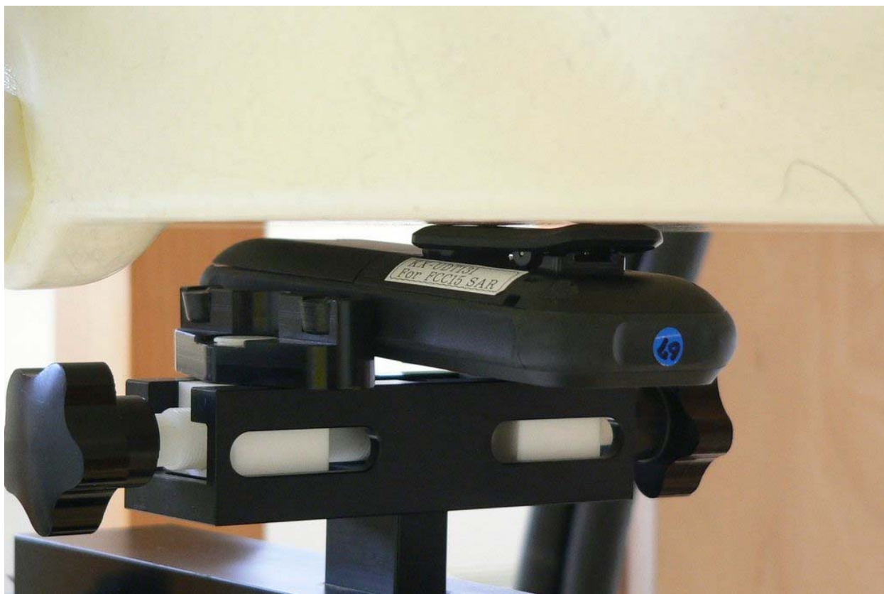
Fig.20: Body worn configuration for KX-UDT131, position 2, display towards the ground, 0 mm distance.
