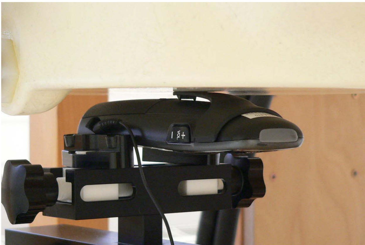
Fig. 21: Body worn configuration KX-TGA470, position 2, display towards the ground, belt clip and headset attached, 0 mm distance.
