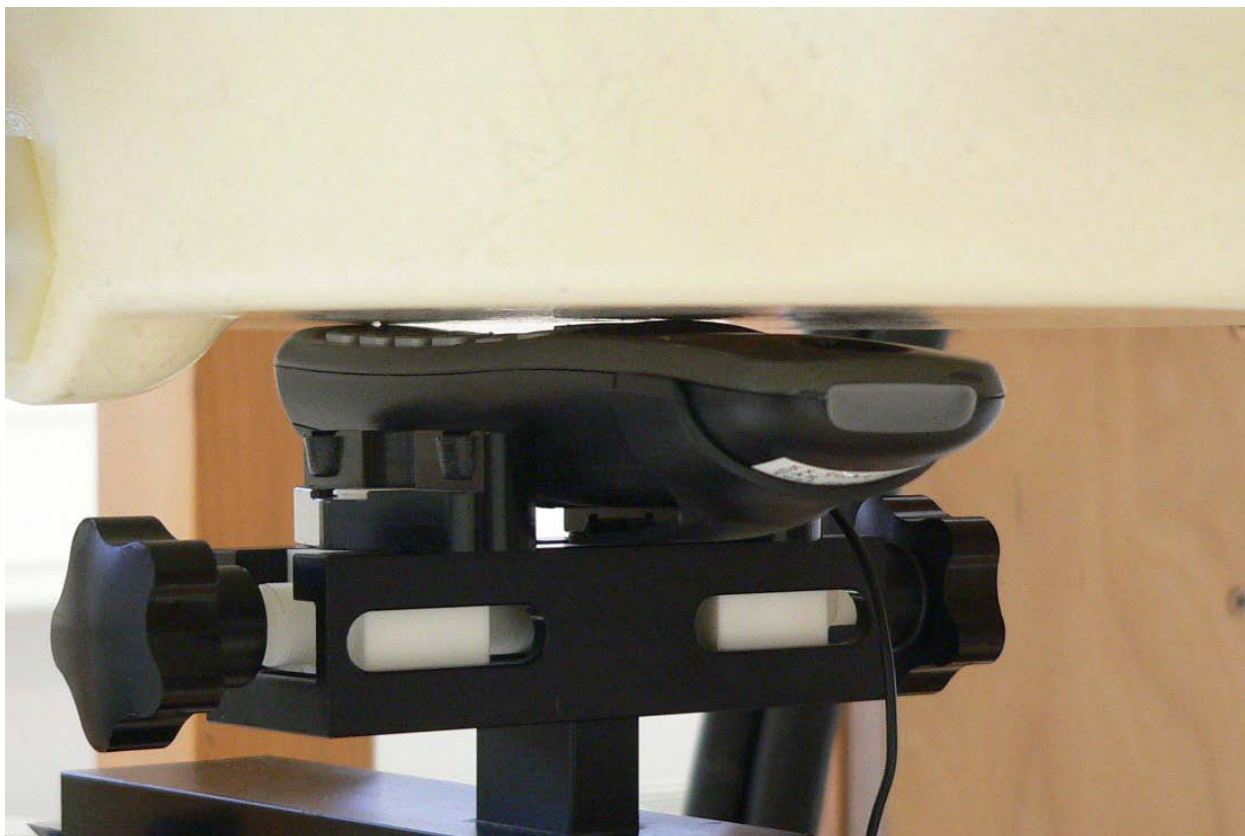
Fig. 20: Body worn configuration KX-TGA470, position 1, display towards the phantom, belt clip and headset attached, 0 mm distance.
