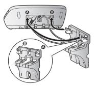
**4** Adjust the adaptor to hold the base unit, then push it in the direction of the arrow until it clicks into place.
