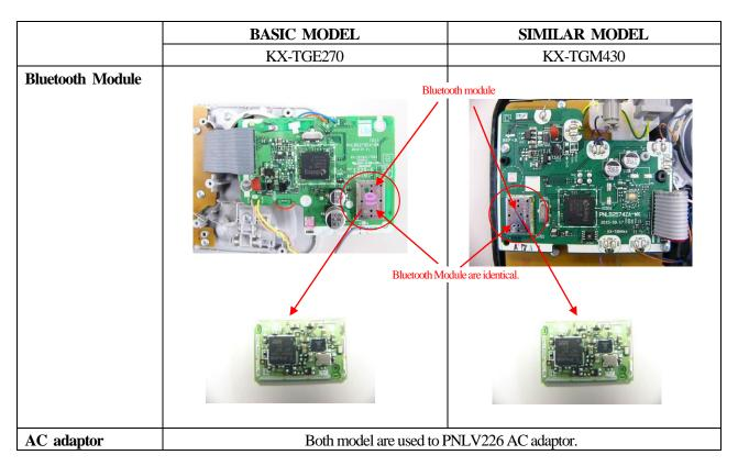
We declare that the Bluetooth module of KX-TGM430 and KX-TGE270 are identical. Regarding the test with conducted of FCC part 15.247 (2.4GHz Frequency Hopping Transmitter), the test of KX-TGM430 are packaged for the test of KX-TGE270 with the following items.
