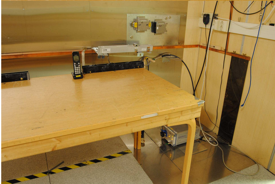
Power-Line Conducted Emissions Test
