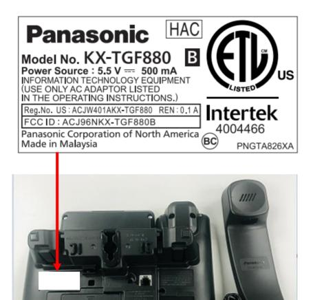
The marking will be shown on lower compartment of the base unit.
