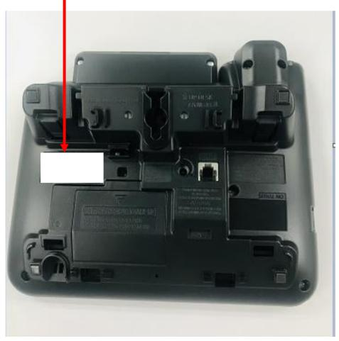
The marking will be shown on lower compartment of the base unit.
