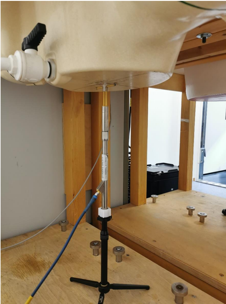
Figure 3 system setup. In system check the DUT is replaced by a verification dipole.
