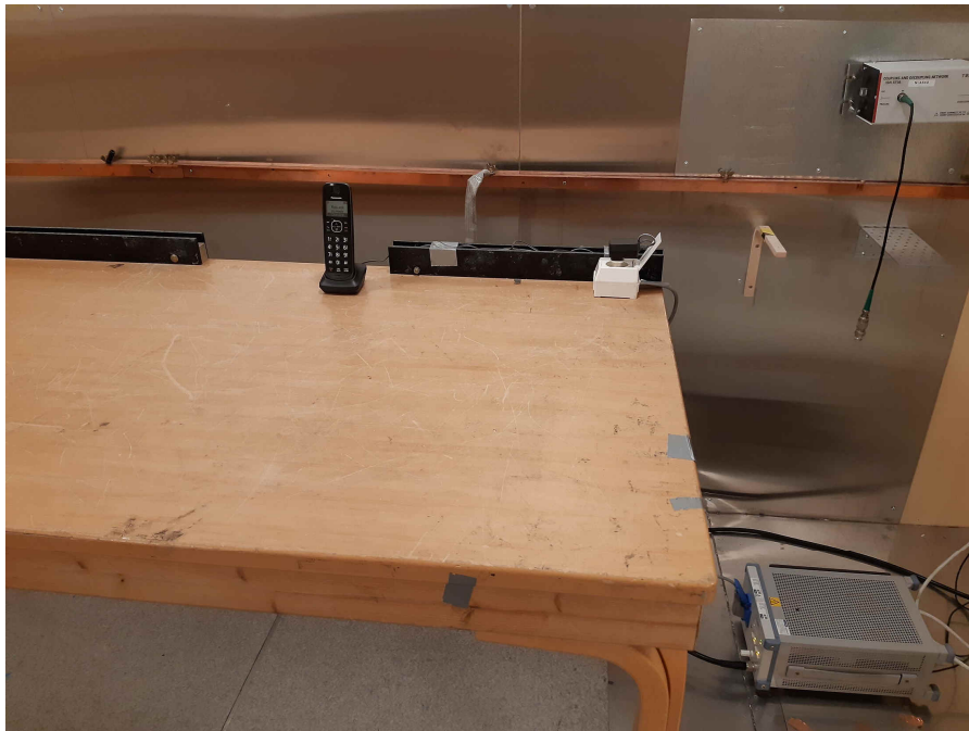
Power-Line Conducted Emissions, Charging
