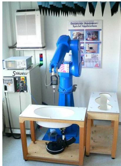
Fig. 3: The measurement set-up with a DASY system and phantoms containing tissue simulating liquid.
