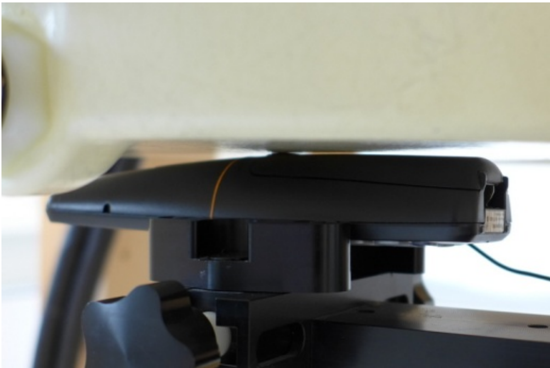
Fig. 20: Body worn configuration for KX-TGEA20, back of the device towards the phantom, headset attached, 0 mm distance.
