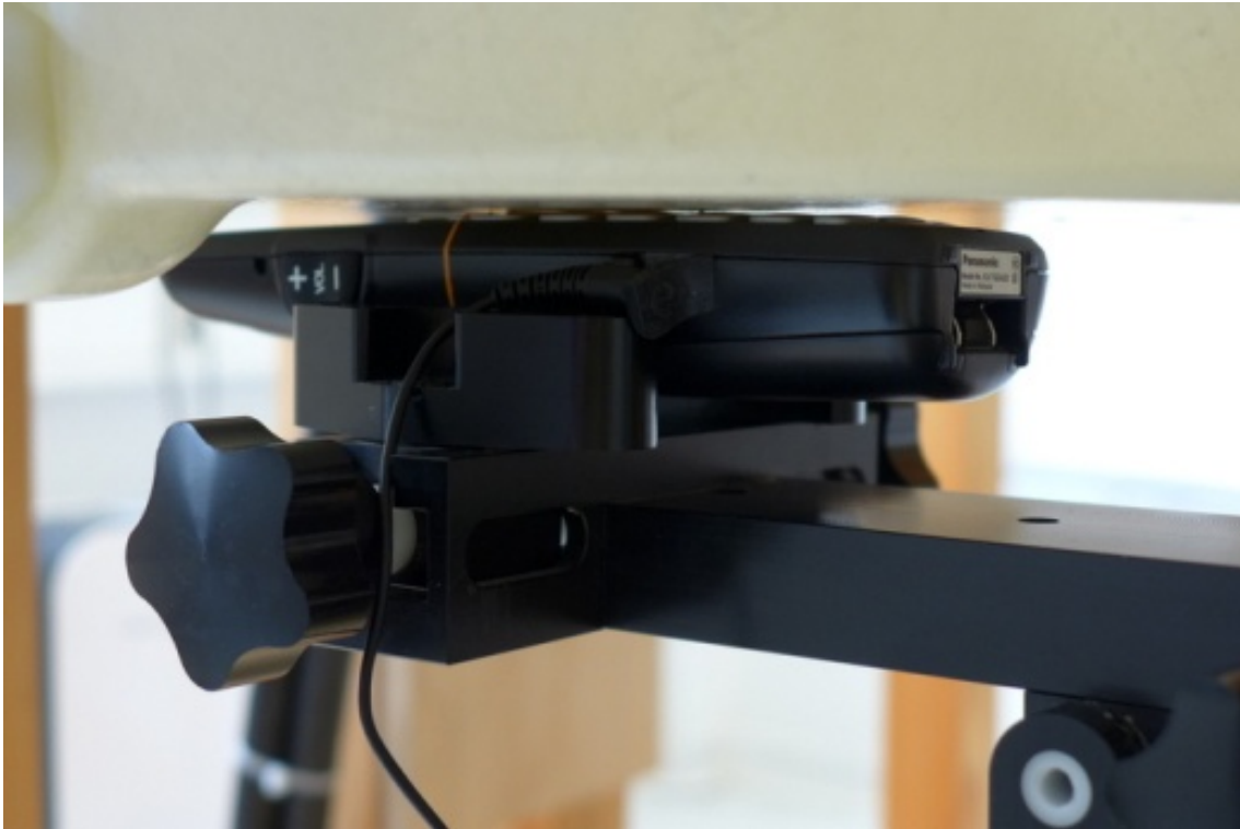
Fig. 19: Body worn configuration for KX-TGEA20, front of the device towards the phantom, headset attached, 0 mm distance.
