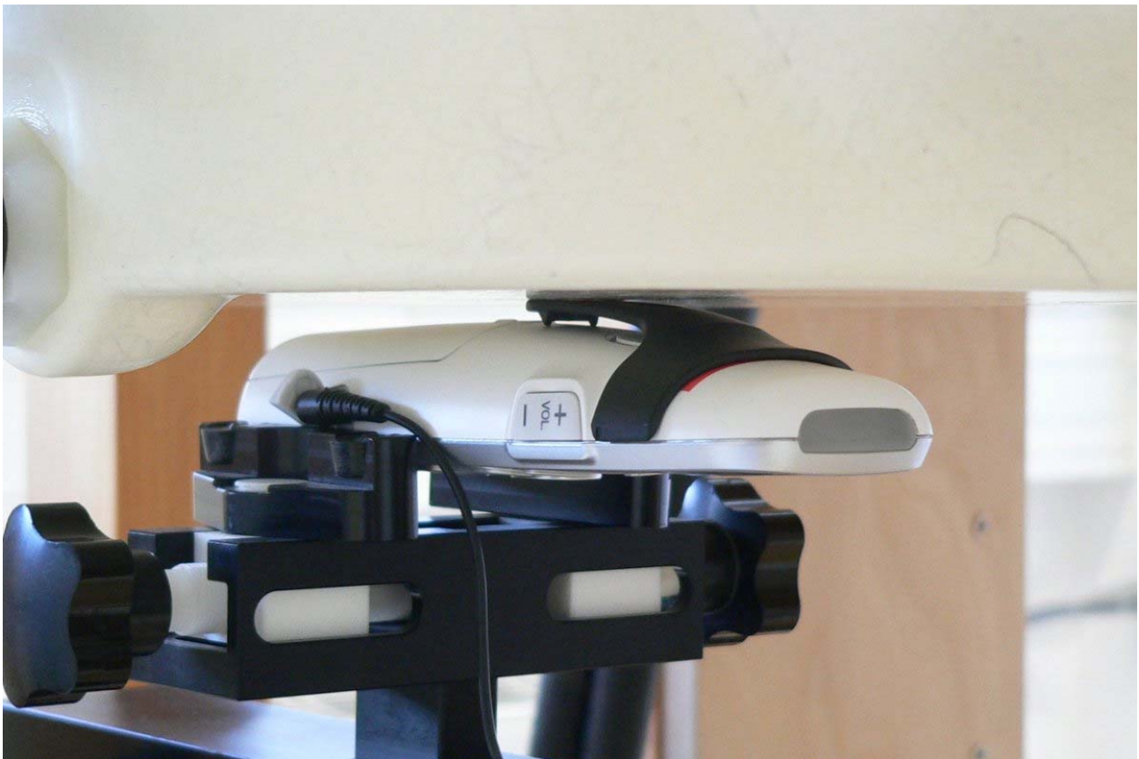
Fig. 20: Body worn configuration for KX-TGAE20, position 2, display towards the ground, headset + belt clip attached, 0 mm distance.
