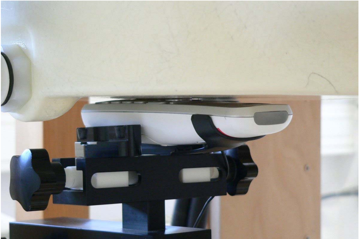
Fig. 19: Body worn configuration for KX-TGAE20, position 1, display towards the phantom, headset + belt clip attached, 0 mm distance.
