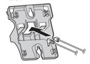
2 Tuck the telephone line cord inside the wall mounting adaptor (1). Connect the AC adaptor cord and telephone line cord
