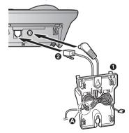
3 Insert the hooks on the wall mounting adaptor into holes (((a)) and ((b)) on the base unit.
