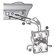
3 Insert the hooks on the wall mounting adaptor into holes (((a)) and ((3)) on the base unit.
