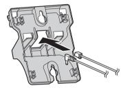
Tuck the telephone line cord inside the wall mounting adaptor (1). Connect the AC adaptor cord and telephone line cord (2).
