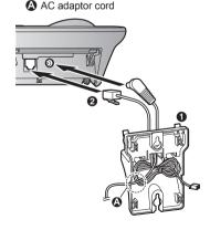
3 Insert the hooks on the wall mounting adaptor into holes (((a)) and ((b)) on the base unit.
