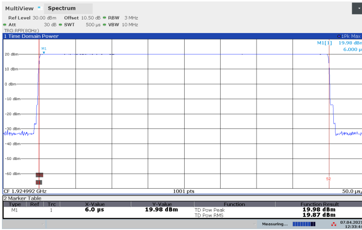
Conducted Peak Output Power, Middle Channel
