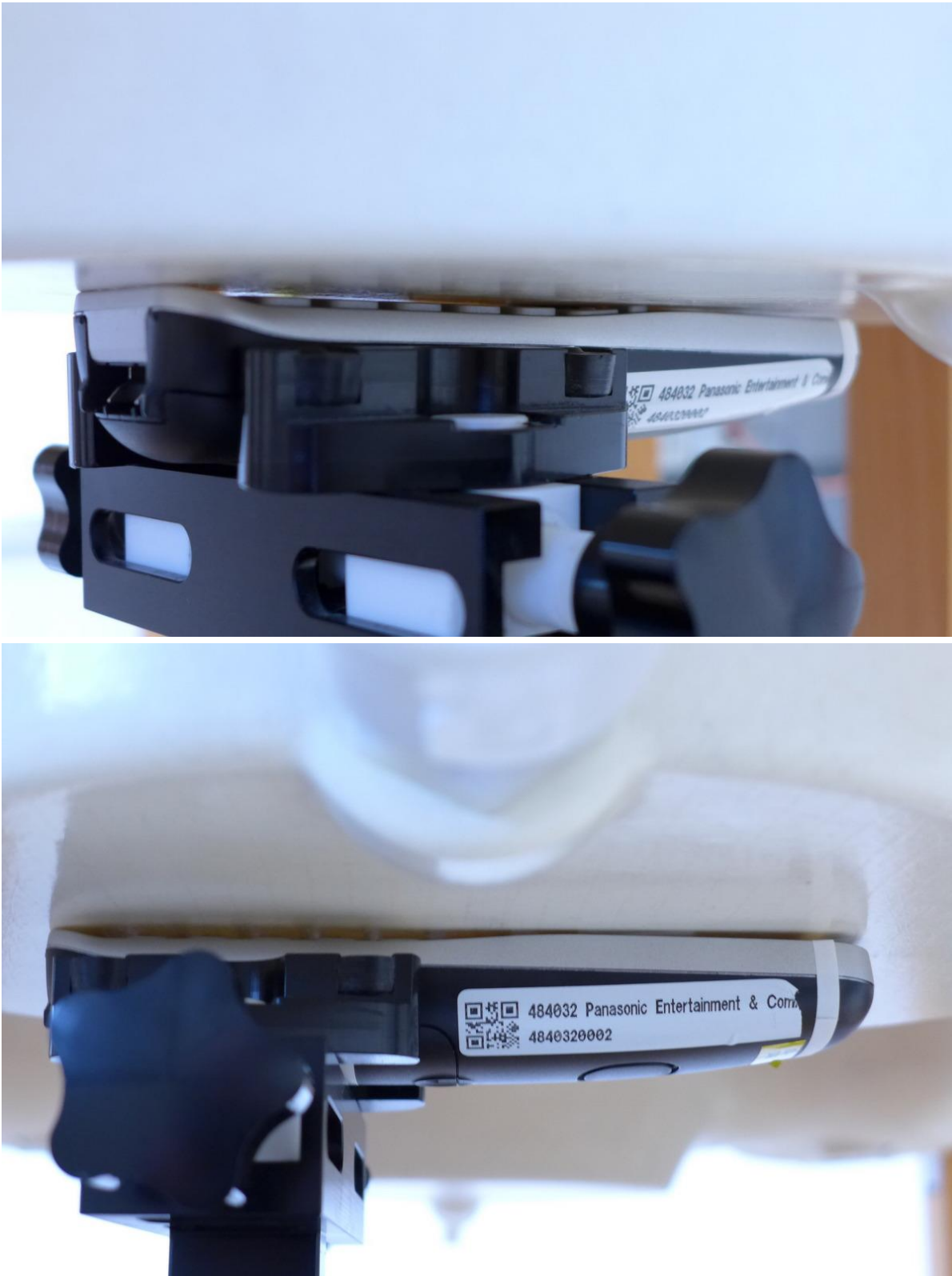
Pic. 7: Test position front side of DUT towards the phantom, 0 mm gap.
