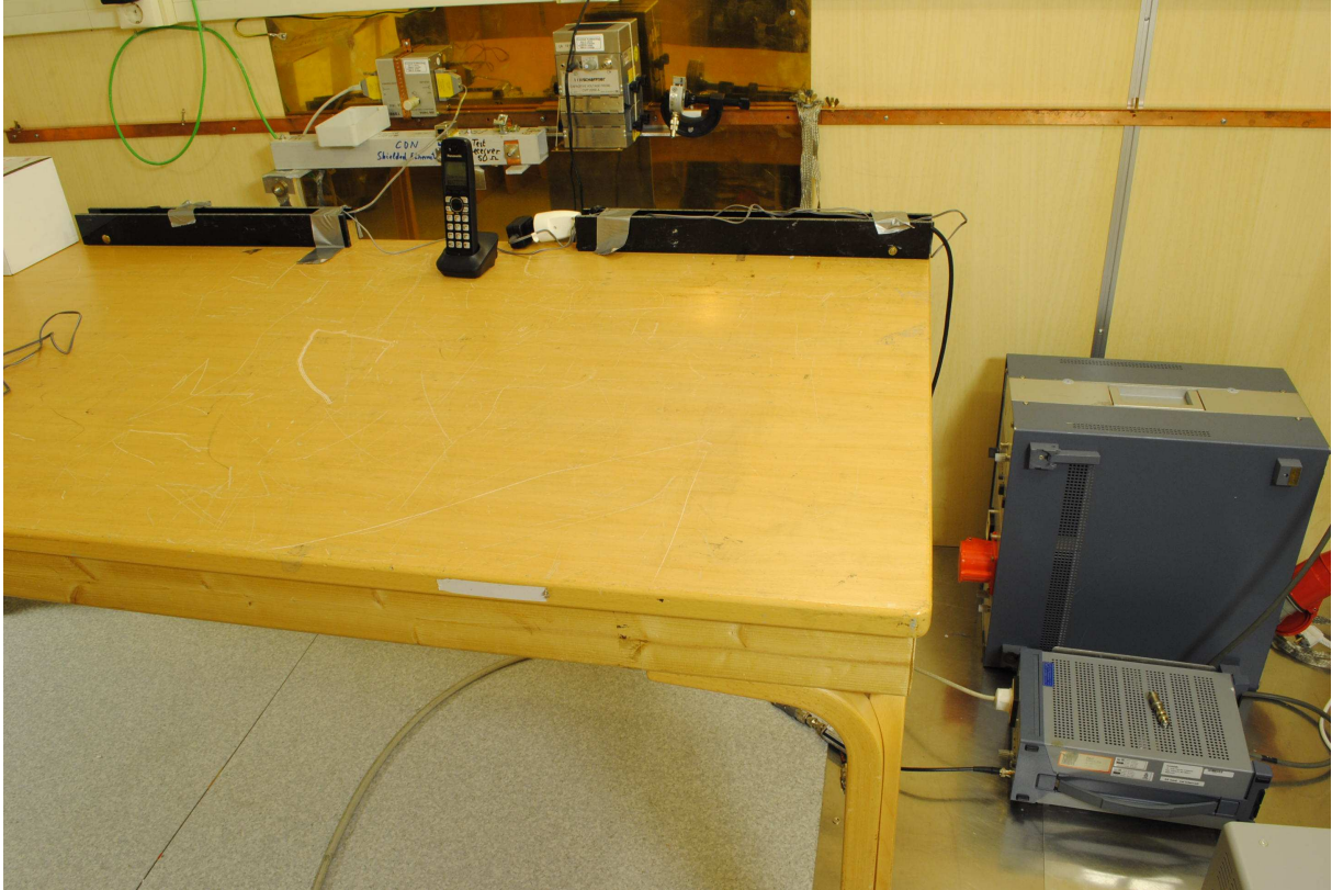
Power line Conducted Emissions Test Set-up
