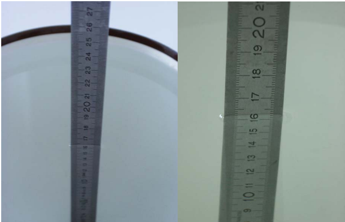
Fig. 22: Liquid depth for 1900 MHz Head and Body measurements.
