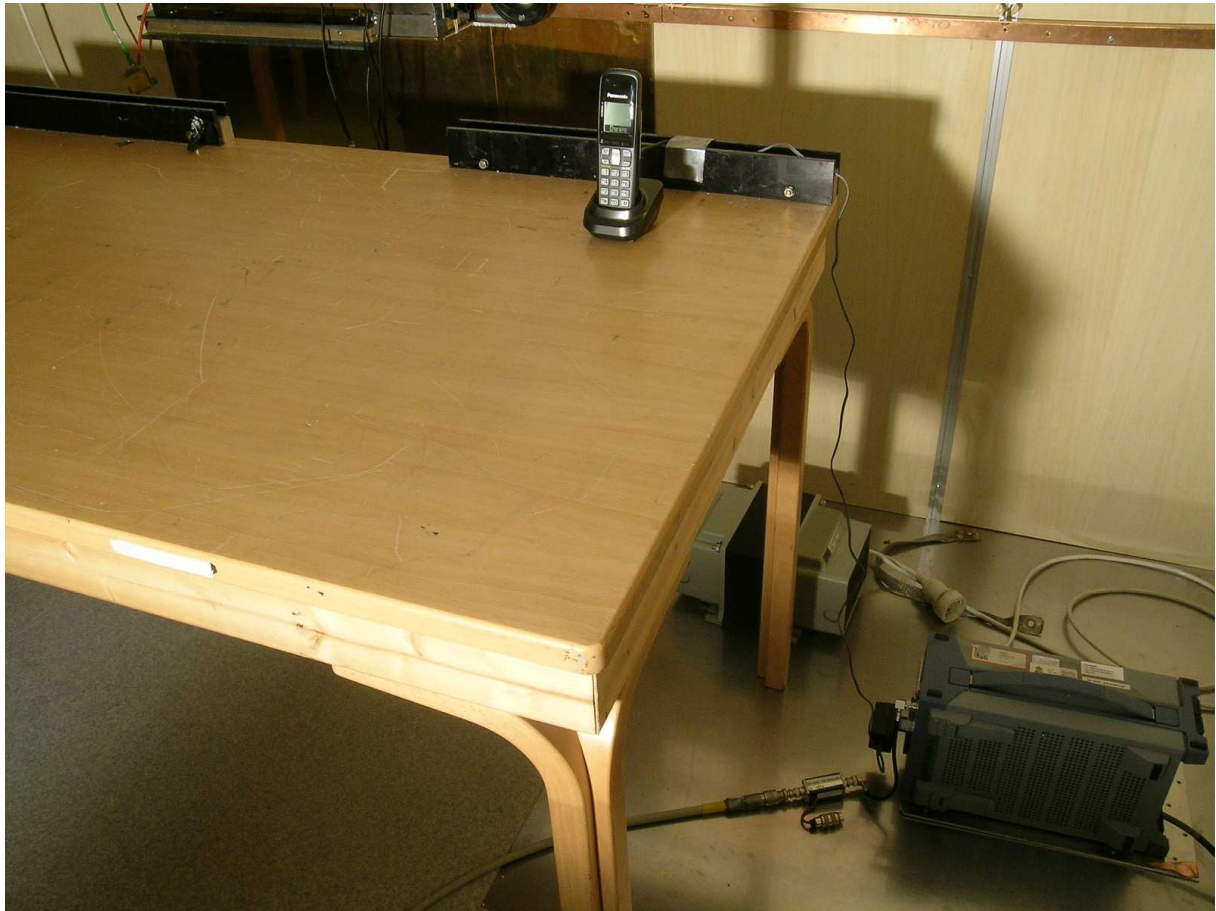
Power-Line Conducted Emissions Test
