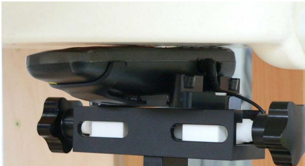
Fig. 20: Body worn configuration, with belt clip and headset, display towards the phantom.
