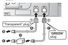
\*DSL/ADSL filter (not supplied) is required if you have DSL/ADSL service.
