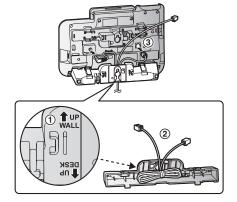
3 Insert the lower tabs of the adaptor into the unit's bottom slots (1), then insert by pushing down the levers of the adaptor into the upper slots (2).
