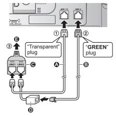
\*DSL/ADSL filter (not supplied) is required if you have DSL/ADSL service.
