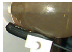
Figure 14. Head SAR Test Setup
