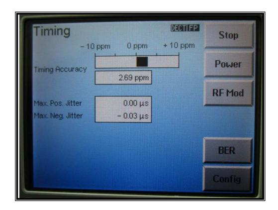
Photo of worst-case of TDMA Frame Jitter display follows:
