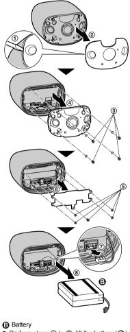
Perform steps ① to ⑧, lift the battery (③), and then remove it.
