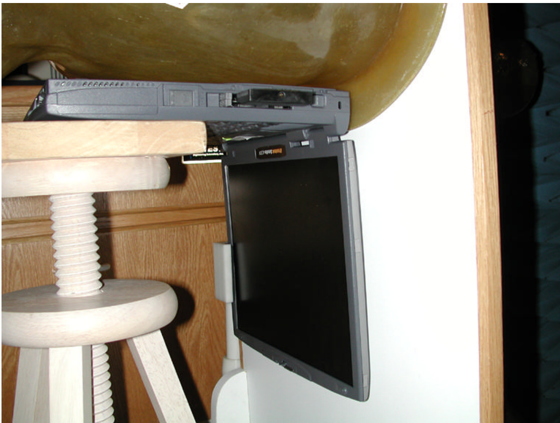
Figure 8. Test setup of EUT in normal operating position with the source of significant emissions (antenna) 1.3 cm below the phantom.
