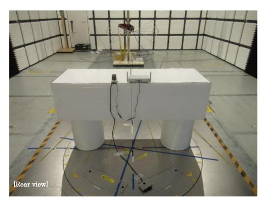
5.2 Radiated Emission, 1 GHz - 6 GHz Test setup in accordance with ANSI C63.4 -2014
