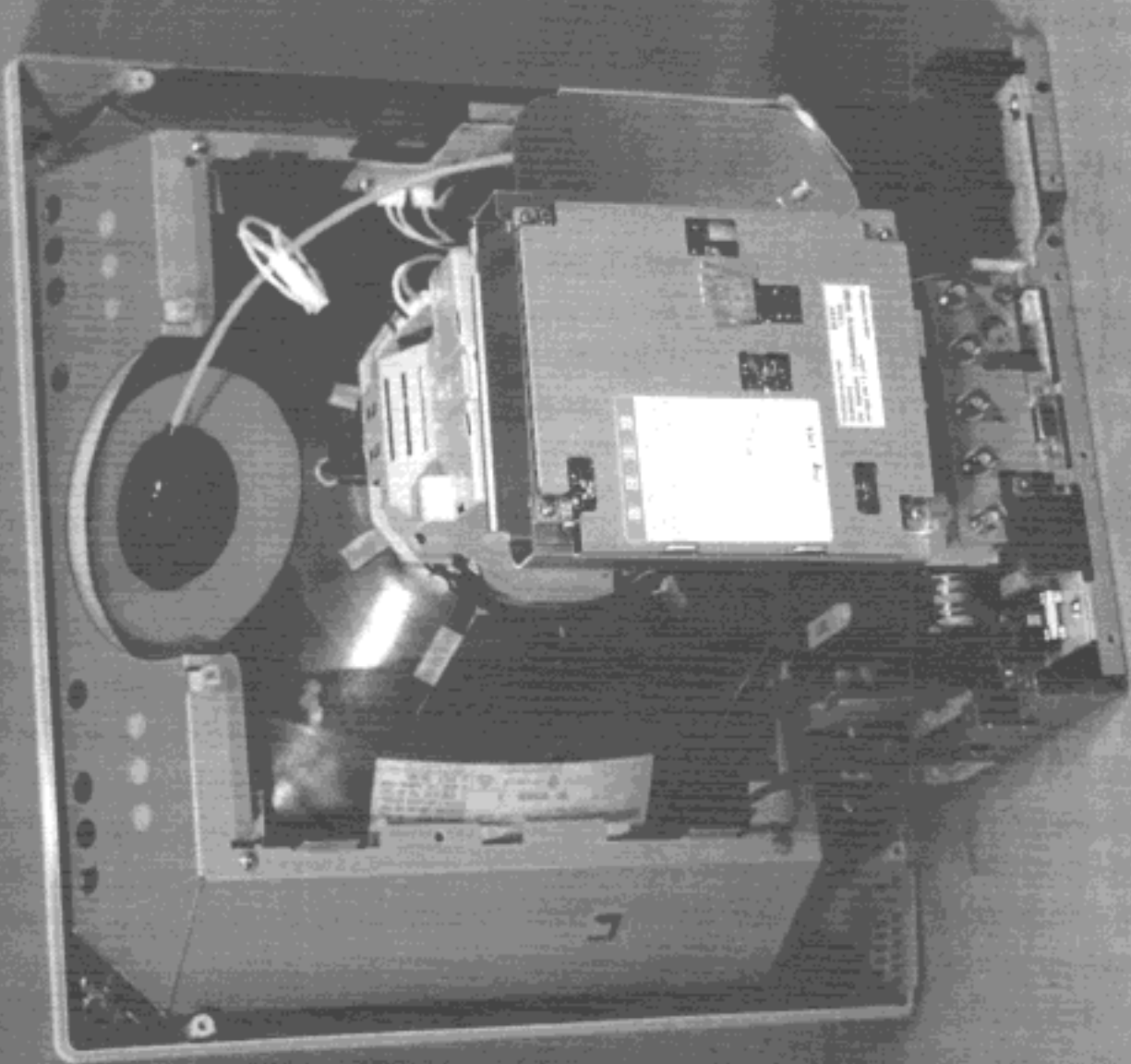
Photo 3. Inside view without shield case of TX-M9T55
