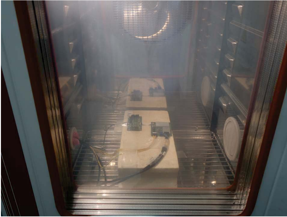
Photograph 3: Set-up for Frequency Tolerance, Inside Temperature Chamber
