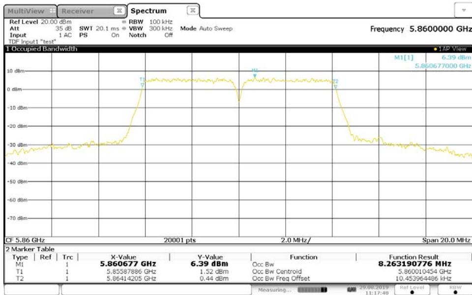
Figure 8: 99% Bandwidth, Mode A (5860MHz) Configuration 2, RF output port 1
