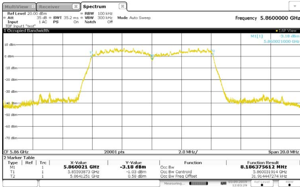
Figure 7: 99% Bandwidth, Mode A (5860MHz) Configuration 1, RF output port 2
