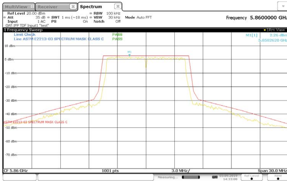
Figure 11: Transmit Spectrum Mask, Mode A (5860MHz) Configuration 2, RF output port 1
