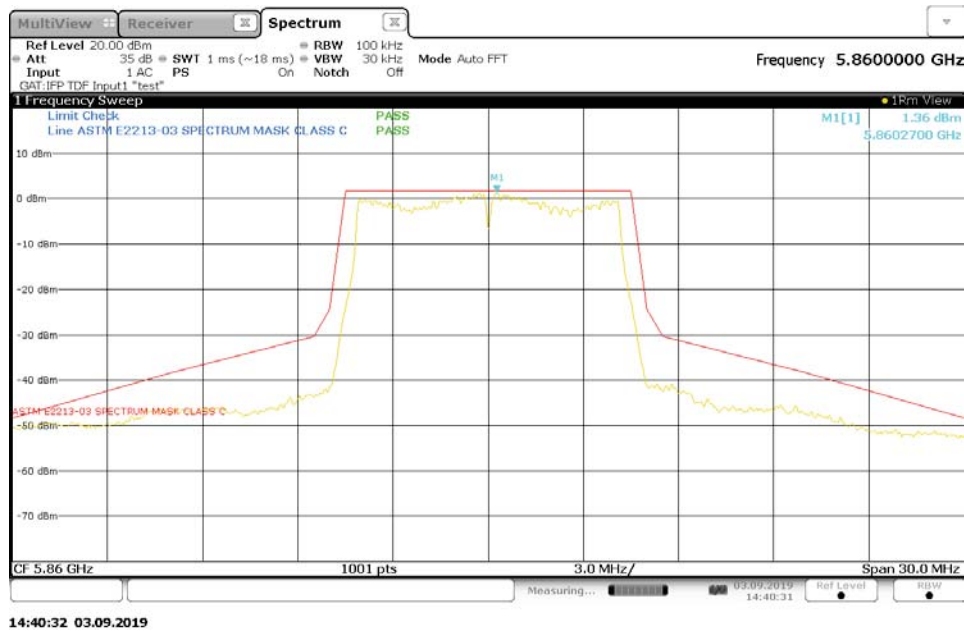
Figure 10: Transmit Spectrum Mask, Mode A (5860MHz) Configuration 1, RF output port 2
