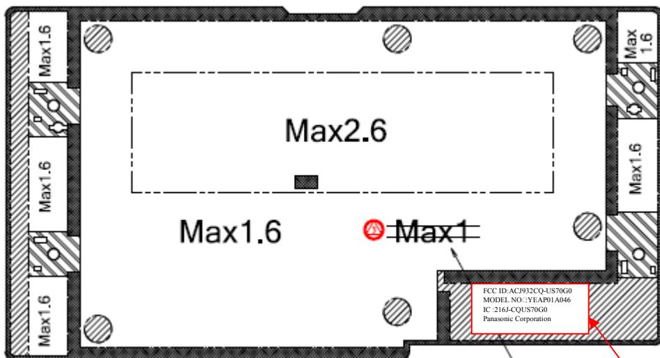
Label must be printed on PCB
