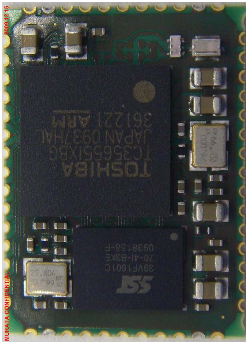
Bluetooth Module TopView without shield
