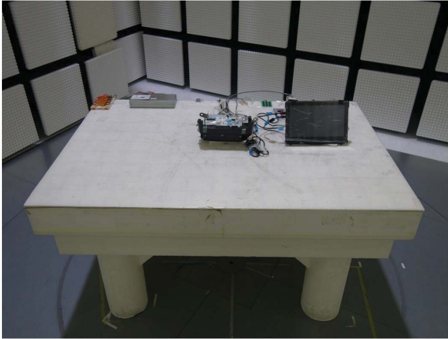
Photograph 2: Set-up for Radiated Emission of Transmitter at MHz Range, Rear View
