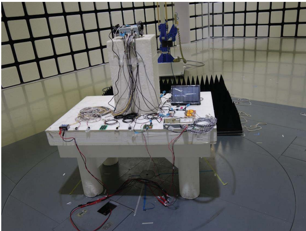
Photograph 4: Set-up for Radiated Emission of Transmitter at GHz Range, Rear View
