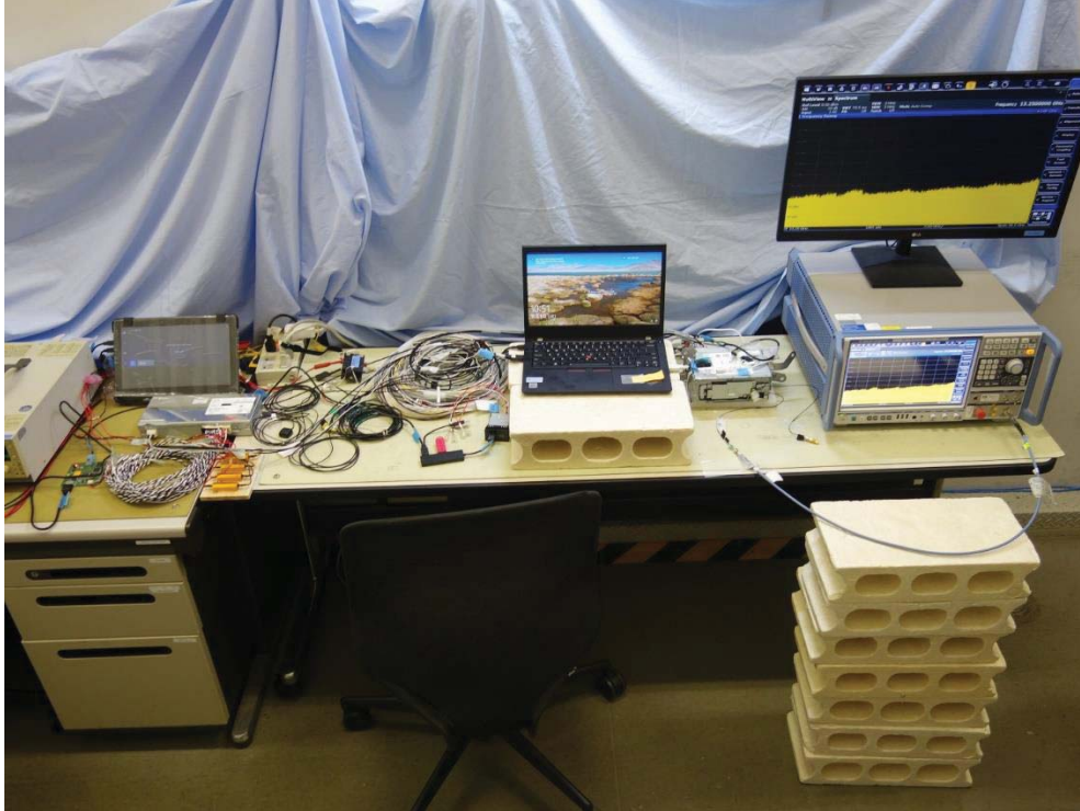
Photograph 5: Set-up for Antenna Port Connected Test
