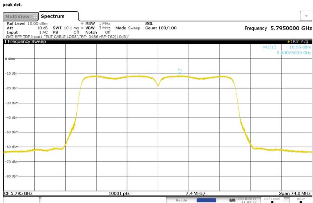
Figure 250: Maximum Power Spectral Density, 802.11ac-40, CDD, RF0, 5795MHz
