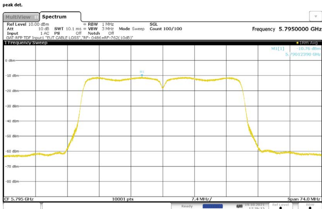
Figure 262: Maximum Power Spectral Density, 802.11ac-40, MIMO, RF1, 5795MHz
