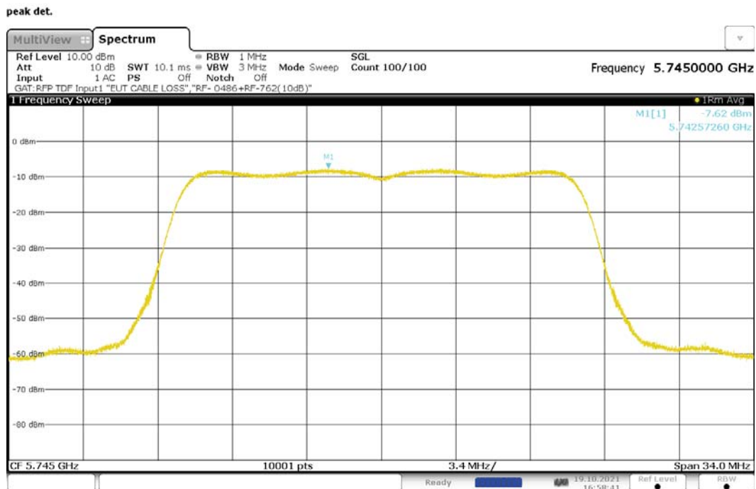
Figure 200: Maximum Power Spectral Density, 802.11ac-20, CDD, RF1, 5745MHz
