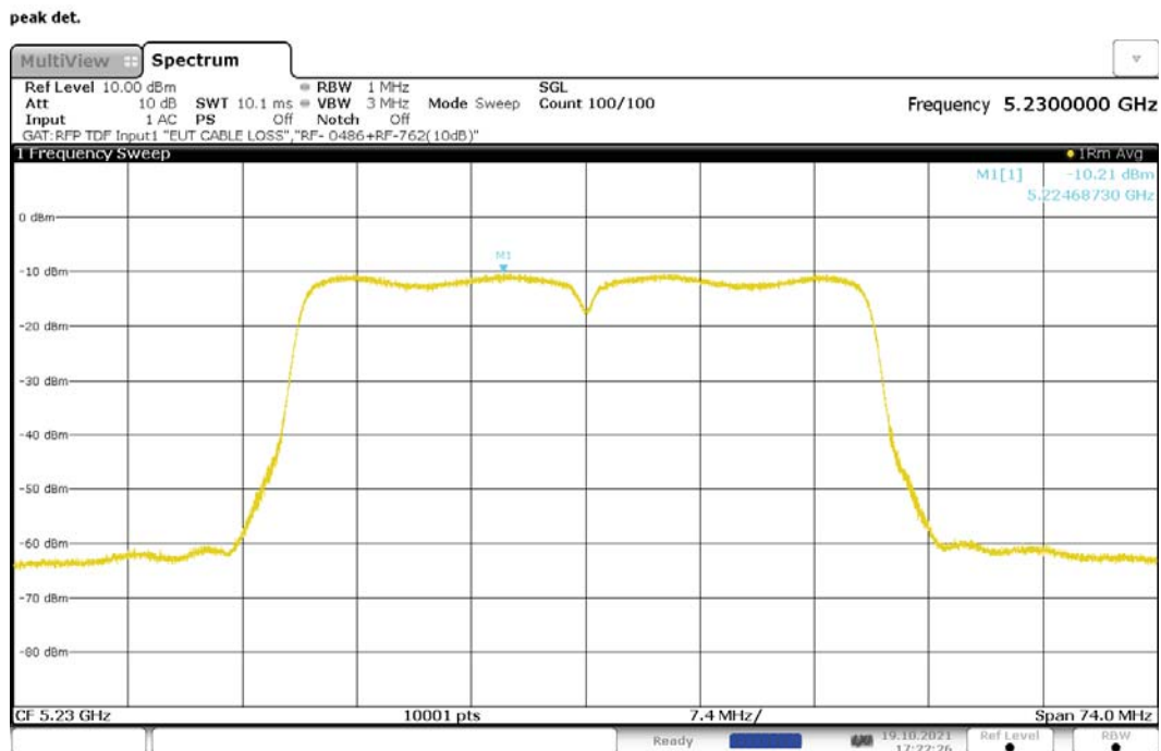
Figure 260: Maximum Power Spectral Density, 802.11ac-40, MIMO, RF1, 5230MHz
