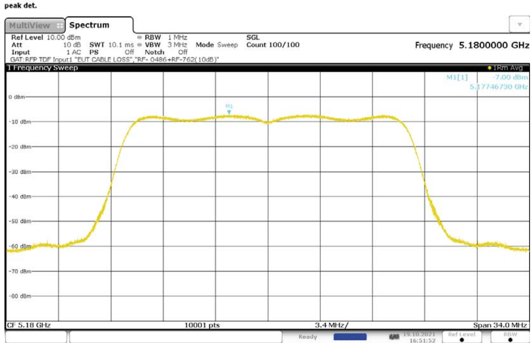
Figure 209: Maximum Power Spectral Density, 802.11ac-20, MIMO, RF1, 5180MHz
