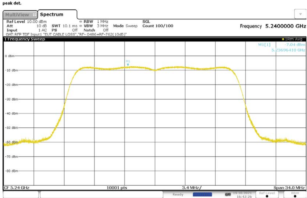
Figure 175: Maximum Power Spectral Density, 802.11n-20, MIMO, RF1, 5240MHz
