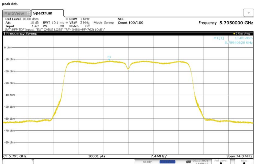
Figure 226: Maximum Power Spectral Density, 802.11n-40, CDD, RF0, 5795MHz
