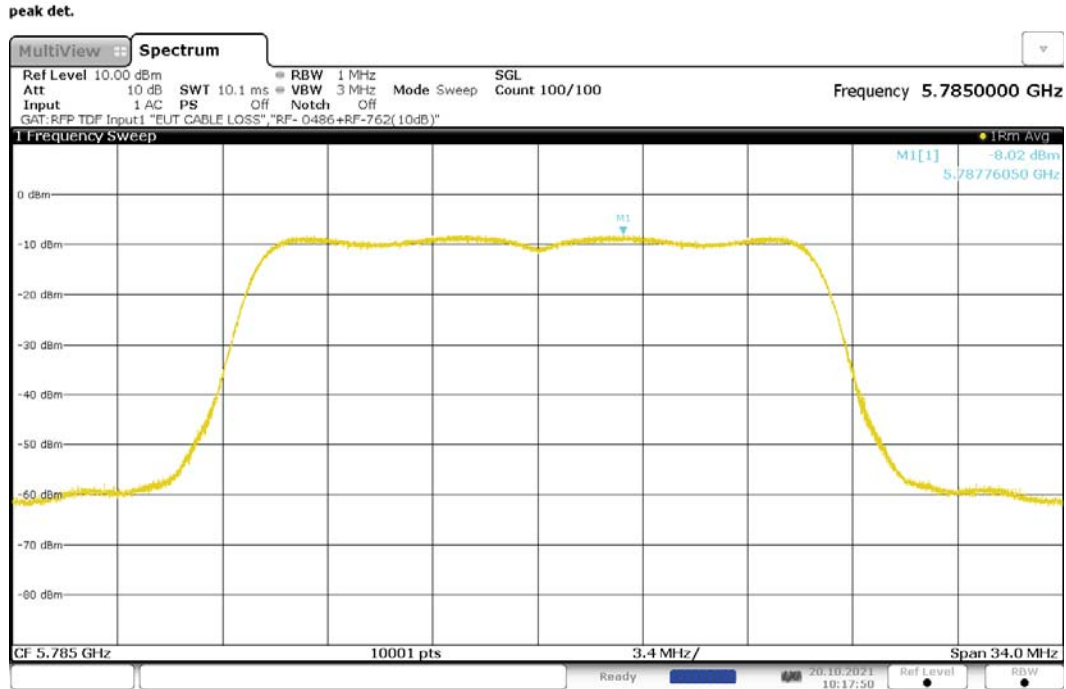
Figure 207: Maximum Power Spectral Density, 802.11ac-20, MIMO, RF0, 5785MHz
