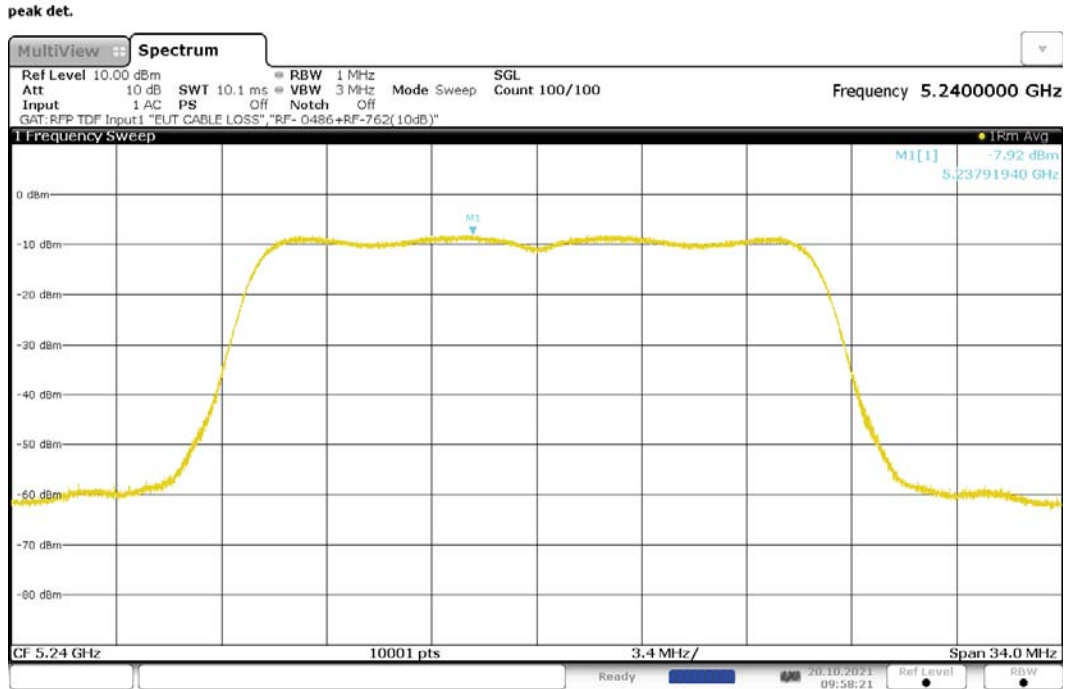
Figure 181: Maximum Power Spectral Density, 802.11ac-20, SISO, RF0, 5240MHz
