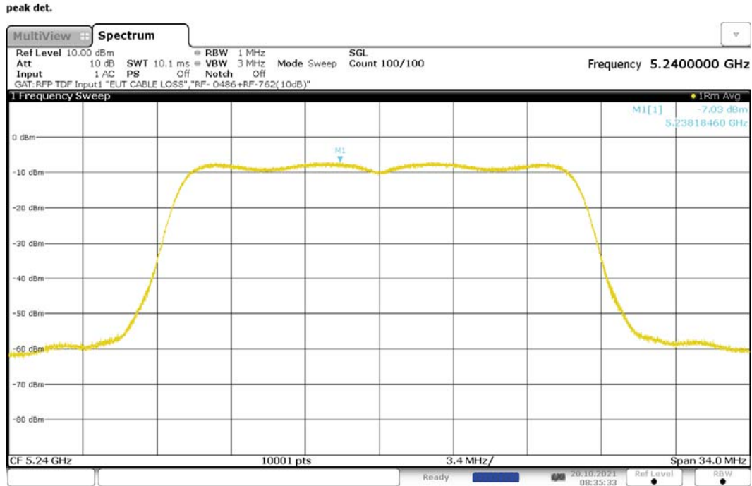
Figure 187: Maximum Power Spectral Density, 802.11ac-20, SISO, RF1, 5240MHz
