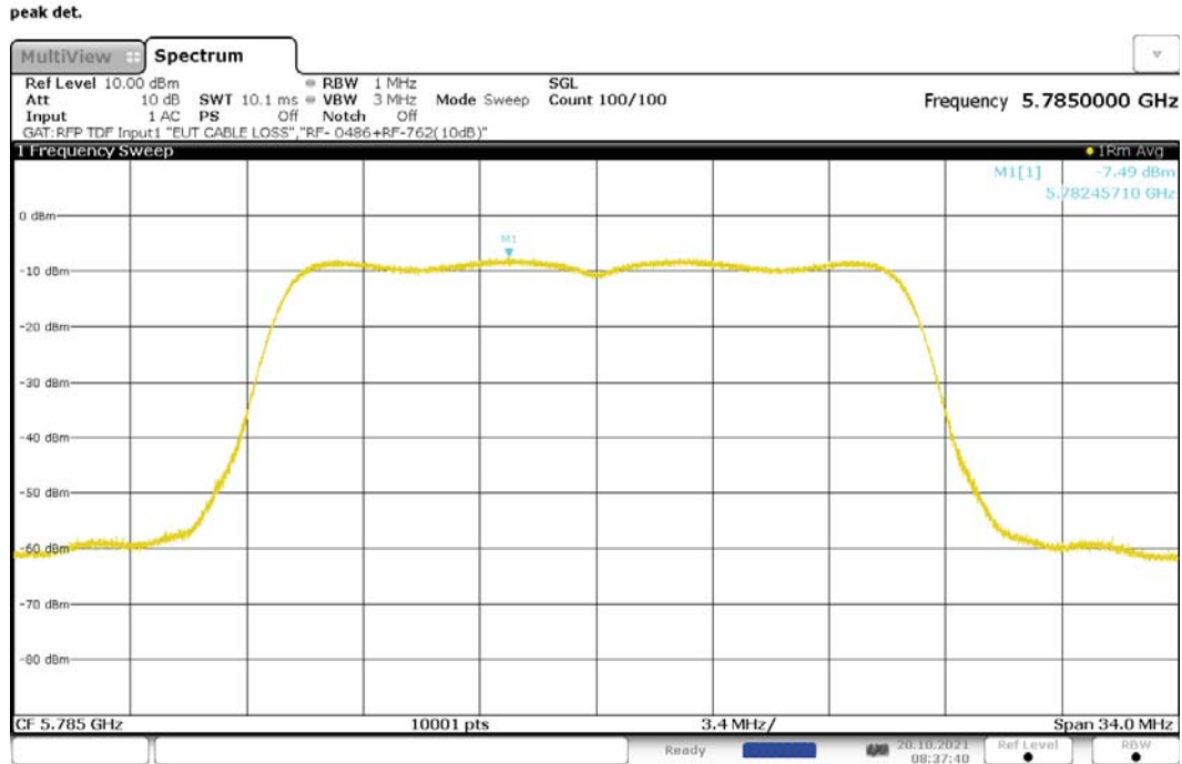
Figure 189: Maximum Power Spectral Density, 802.11ac-20, SISO, RF1, 5785MHz
