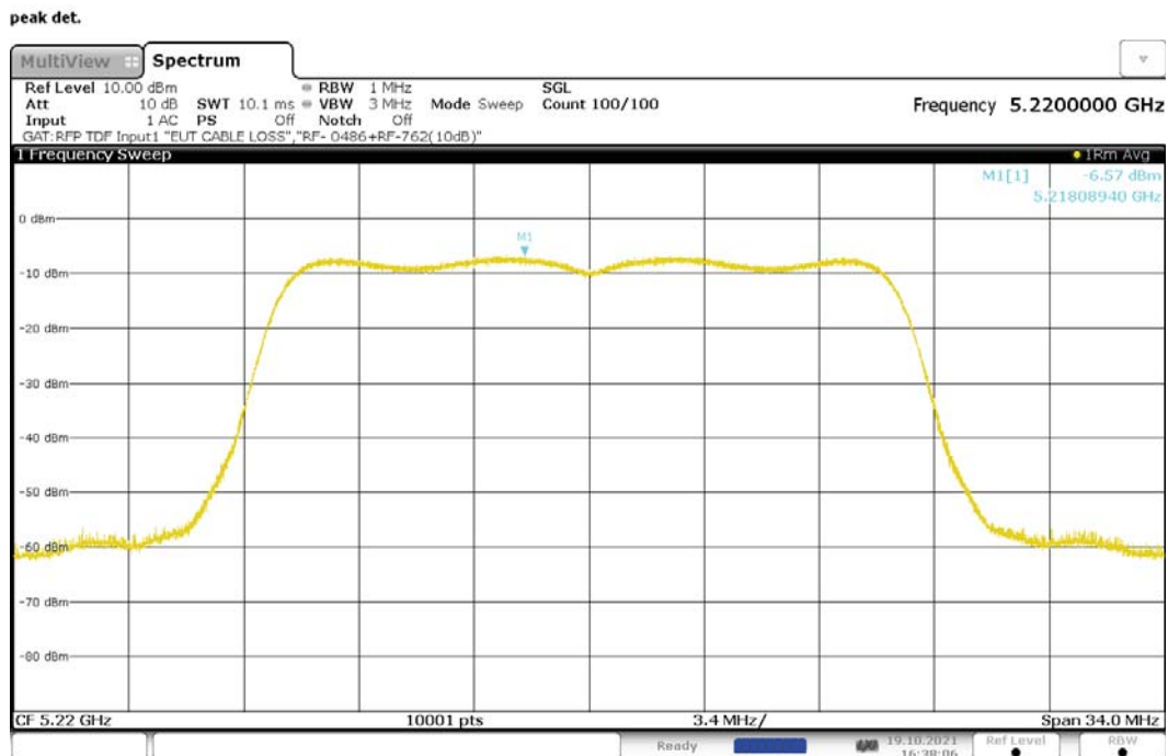
Figure 174: Maximum Power Spectral Density, 802.11n-20, MIMO, RF1, 5220MHz
