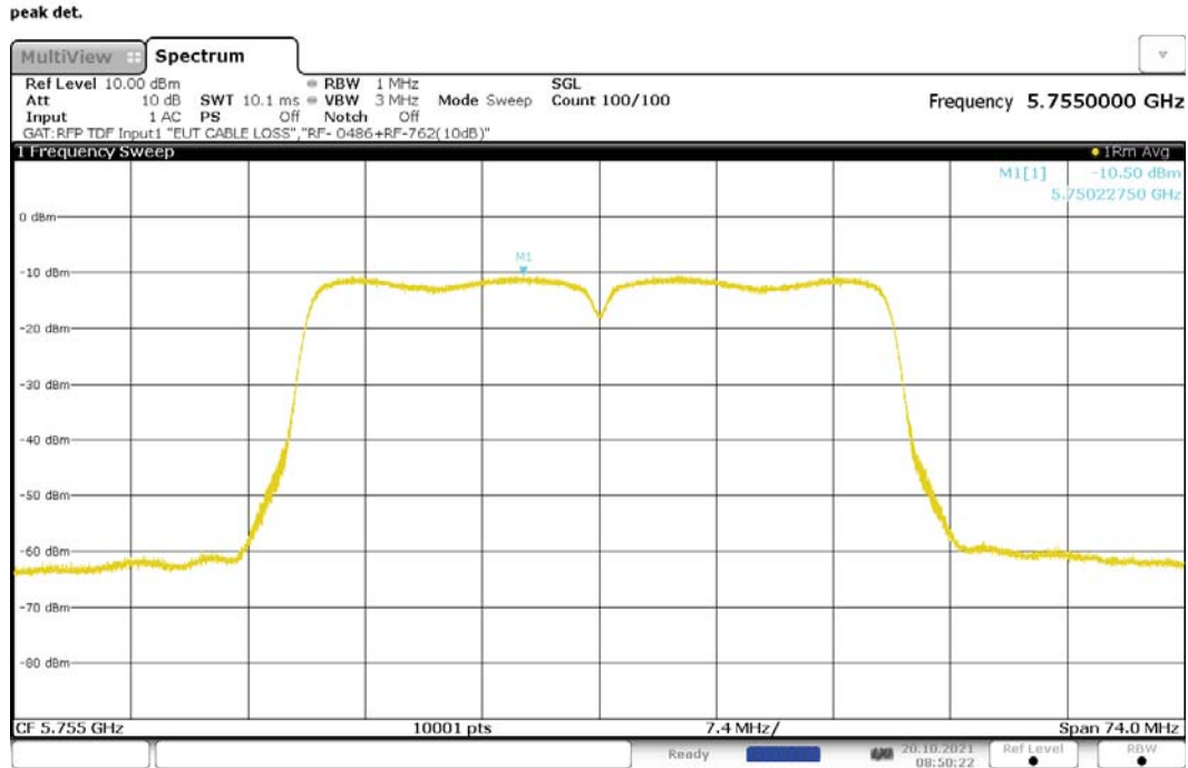
Figure 221: Maximum Power Spectral Density, 802.11n-40, SISO, RF1, 5755MHz
