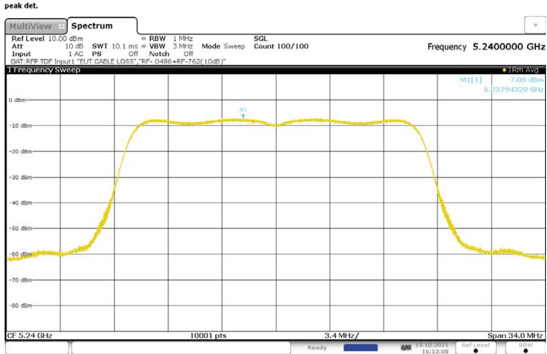
Figure 211: Maximum Power Spectral Density, 802.11ac-20, MIMO, RF1, 5240MHz
