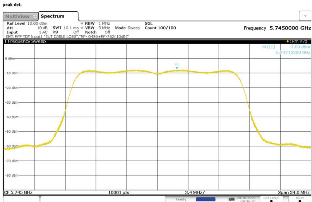
Figure 188: Maximum Power Spectral Density, 802.11ac-20, SISO, RF1, 5745MHz
