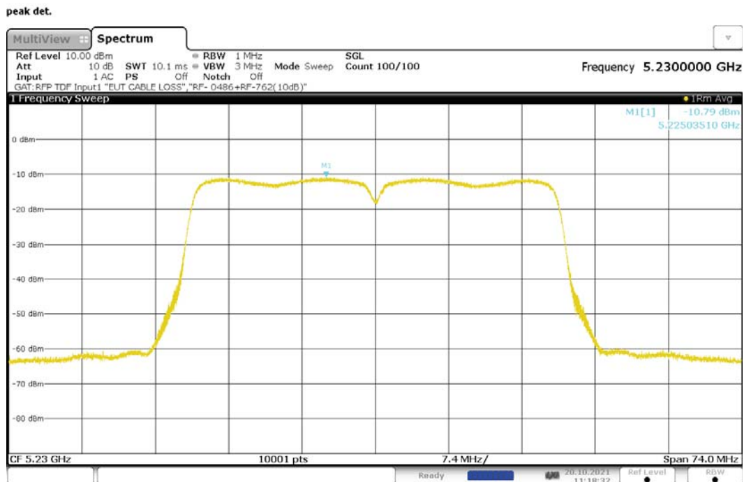
Figure 216: Maximum Power Spectral Density, 802.11n-40, SISO, RF0, 5230MHz
