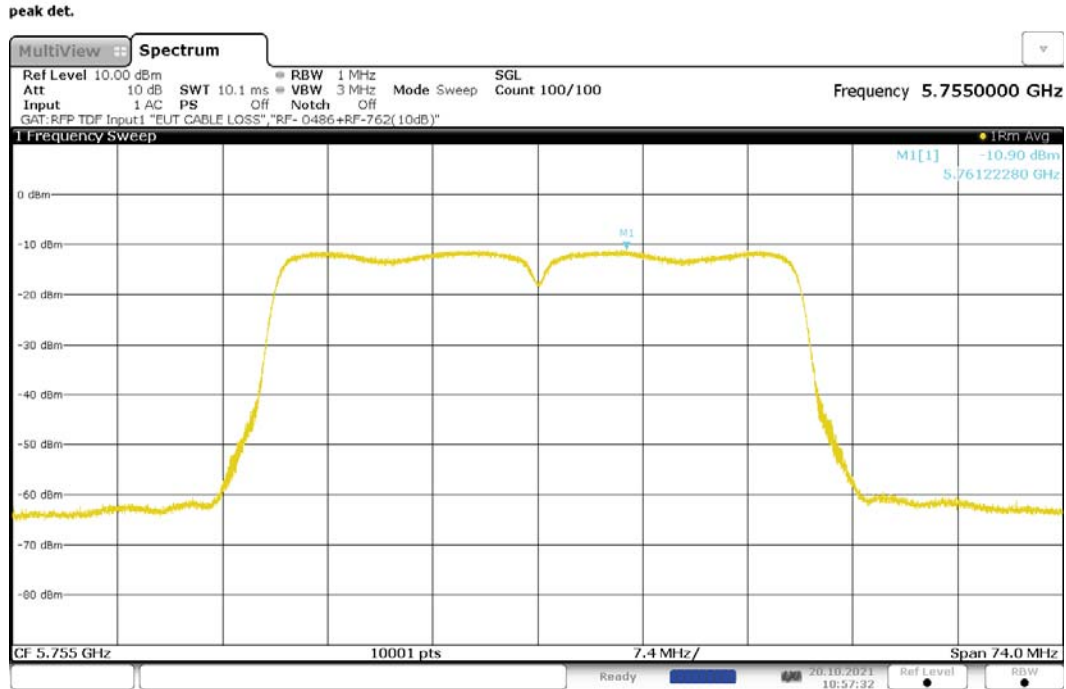
Figure 233: Maximum Power Spectral Density, 802.11n-40, MIMO, RF0, 5755MHz
