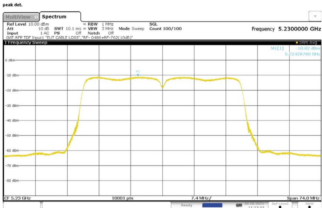
Figure 240: Maximum Power Spectral Density, 802.11ac-40, SISO, RF0, 5230MHz
