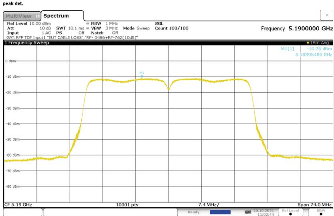
Figure 255: Maximum Power Spectral Density, 802.11ac-40, MIMO, RF0, 5190MHz
