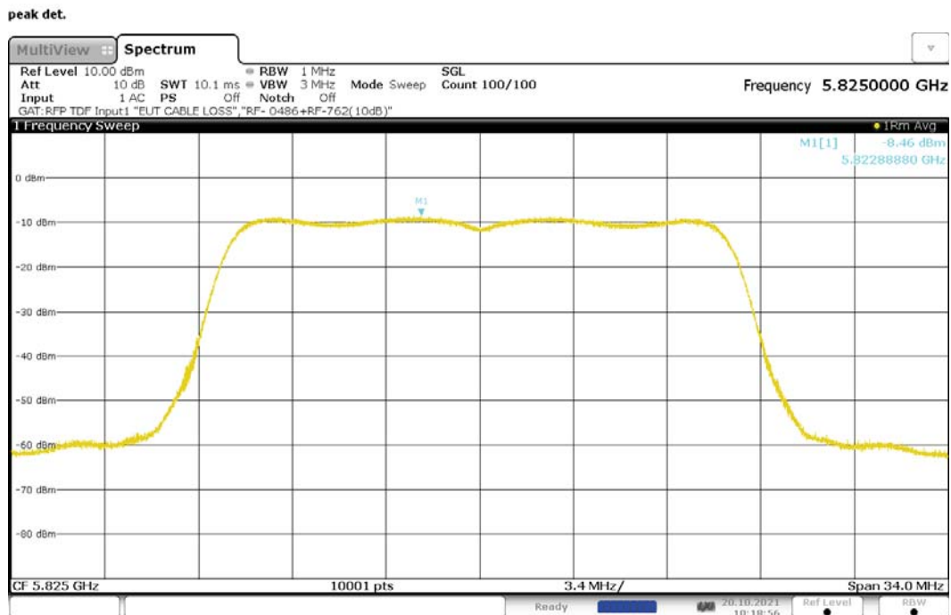
Figure 208: Maximum Power Spectral Density, 802.11ac-20, MIMO, RF0, 5825MHz
