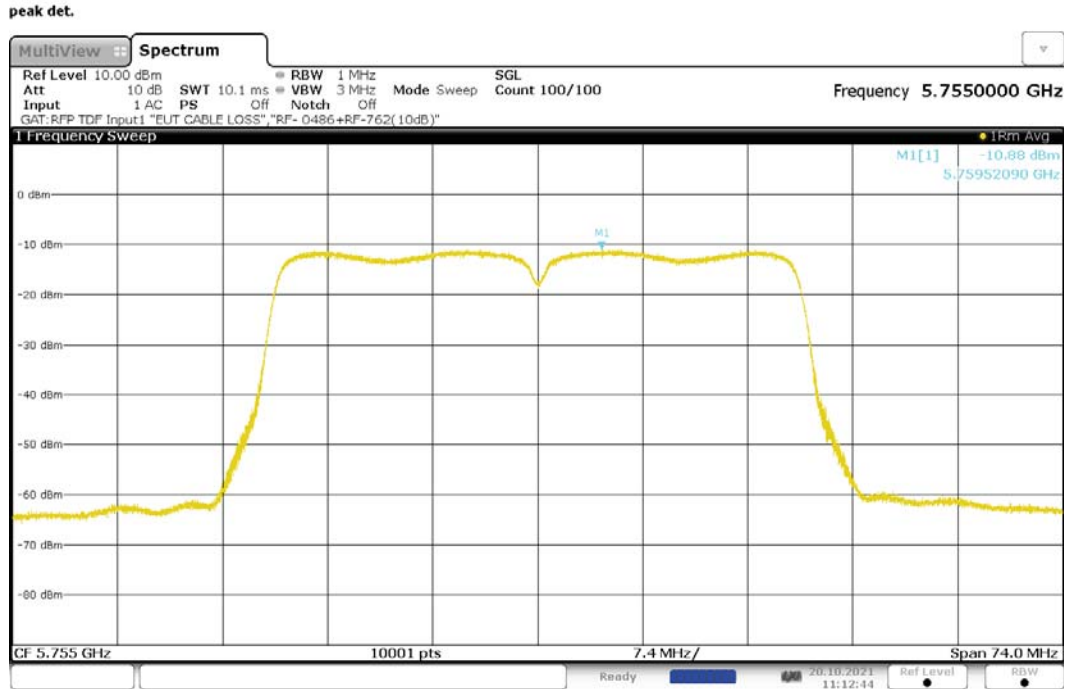
Figure 241: Maximum Power Spectral Density, 802.11ac-40, SISO, RF0, 5755MHz
