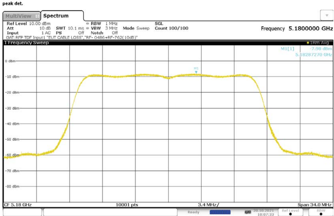
Figure 191: Maximum Power Spectral Density, 802.11ac-20, CDD, RF0, 5180MHz
