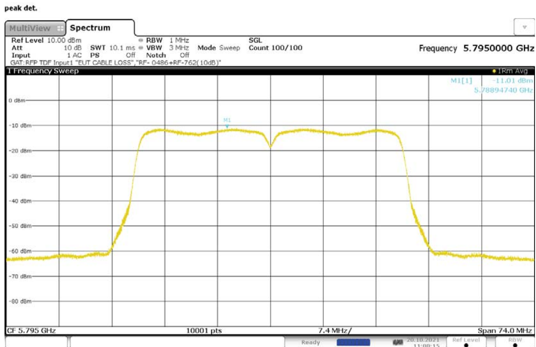
Figure 234: Maximum Power Spectral Density, 802.11n-40, MIMO, RF0, 5795MHz
