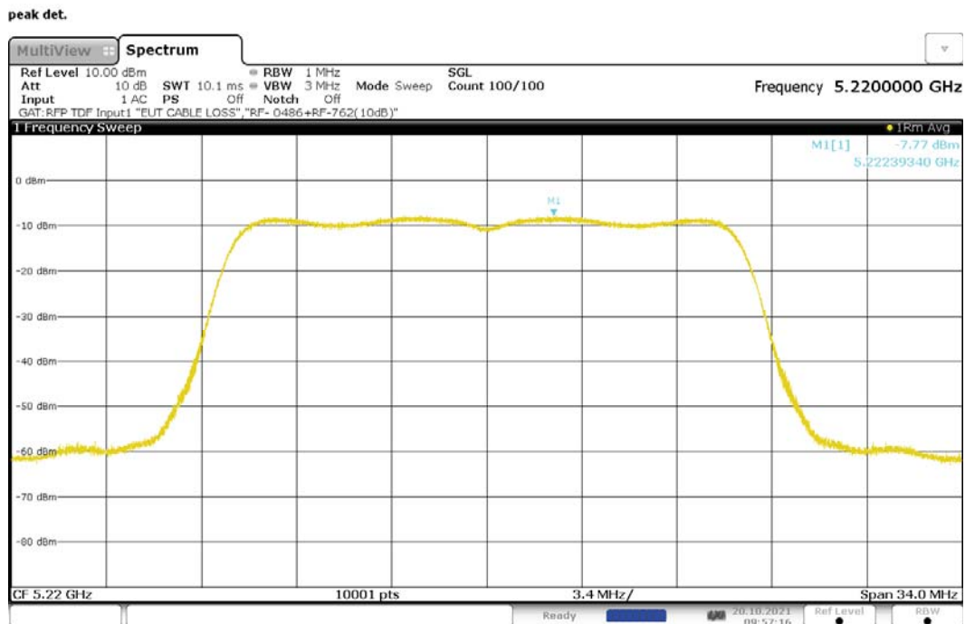
Figure 180: Maximum Power Spectral Density, 802.11ac-20, SISO, RF0, 5220MHz
