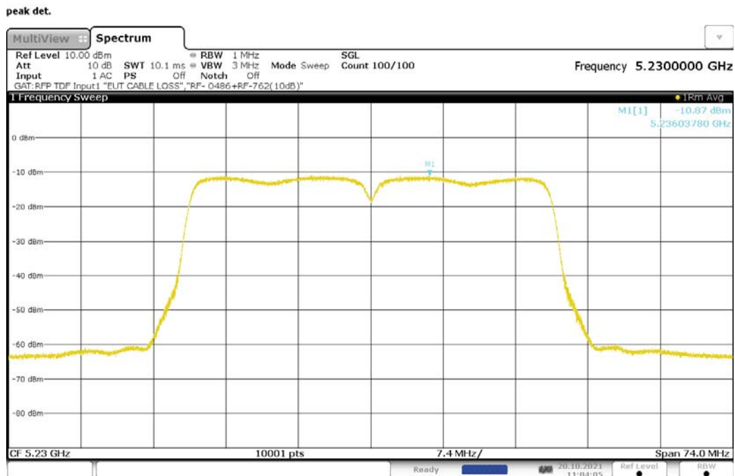
Figure 256: Maximum Power Spectral Density, 802.11ac-40, MIMO, RF0, 5230MHz
