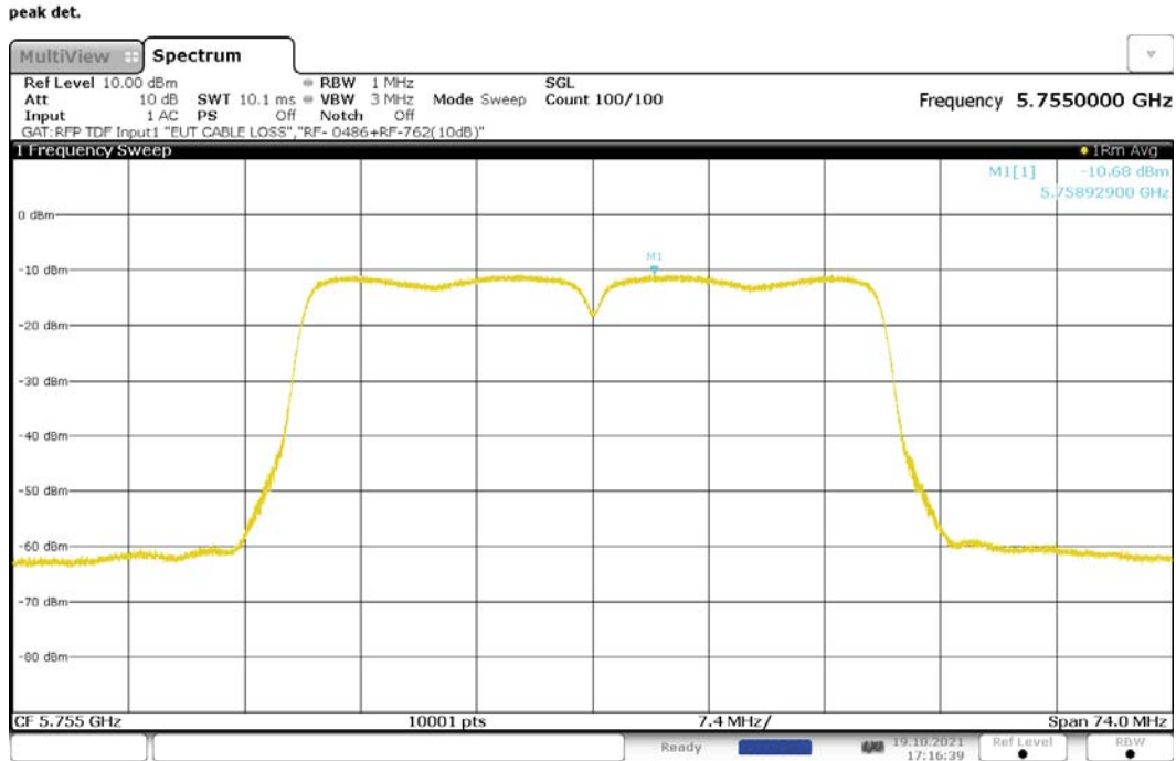
Figure 237: Maximum Power Spectral Density, 802.11n-40, MIMO, RF1, 5755MHz
