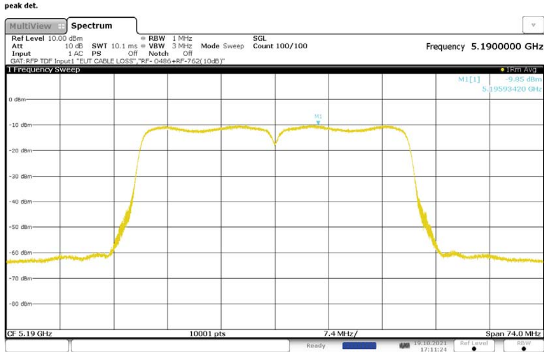
Figure 227: Maximum Power Spectral Density, 802.11n-40, CDD, RF1, 5190MHz
