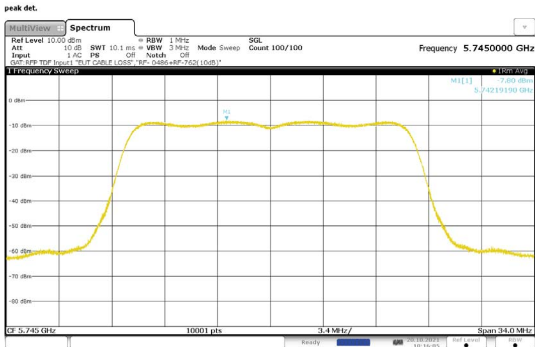
Figure 194: Maximum Power Spectral Density, 802.11ac-20, CDD, RF0, 5745MHz
