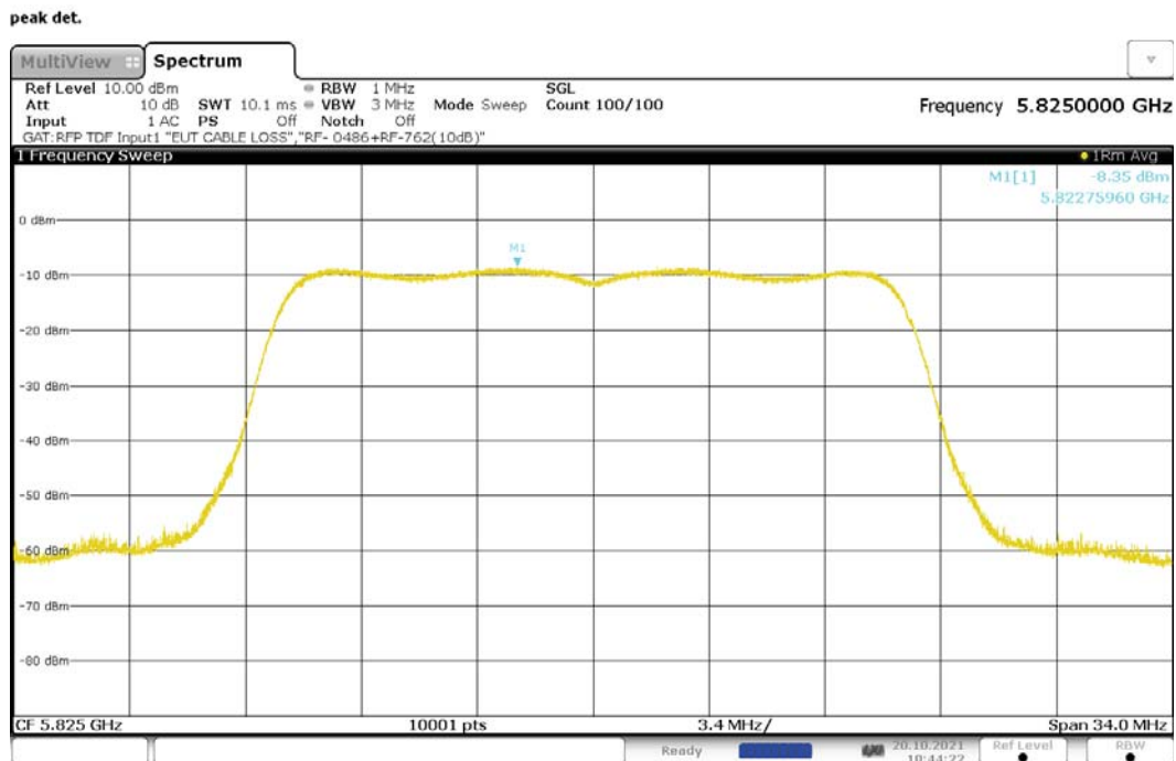
Figure 172: Maximum Power Spectral Density, 802.11n-20, MIMO, RF0, 5825MHz
