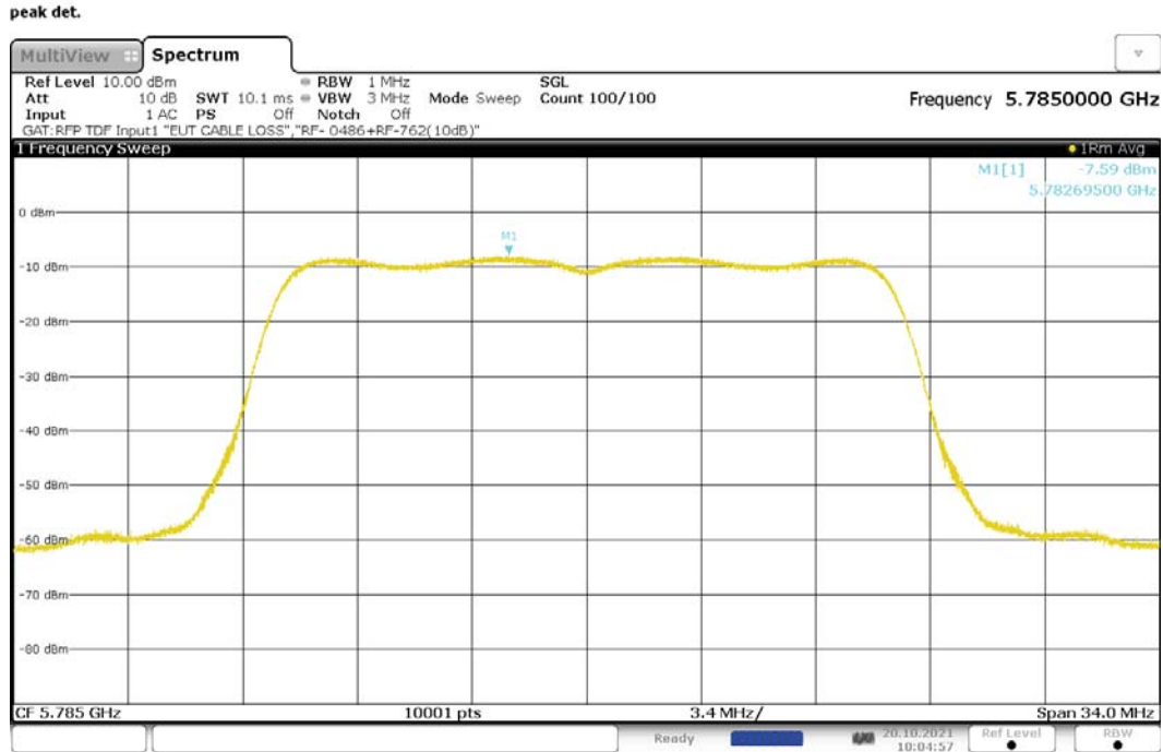
Figure 183: Maximum Power Spectral Density, 802.11ac-20, SISO, RF0, 5785MHz
