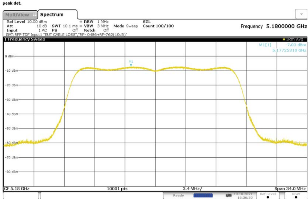
Figure 173: Maximum Power Spectral Density, 802.11n-20, MIMO, RF1, 5180MHz
