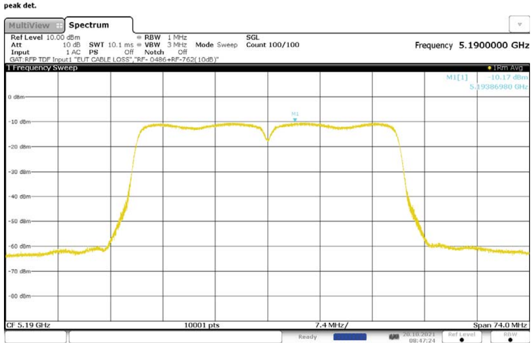
Figure 219: Maximum Power Spectral Density, 802.11n-40, SISO, RF1, 5190MHz
