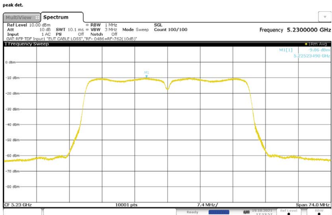
Figure 236: Maximum Power Spectral Density, 802.11n-40, MIMO, RF1, 5230MHz
