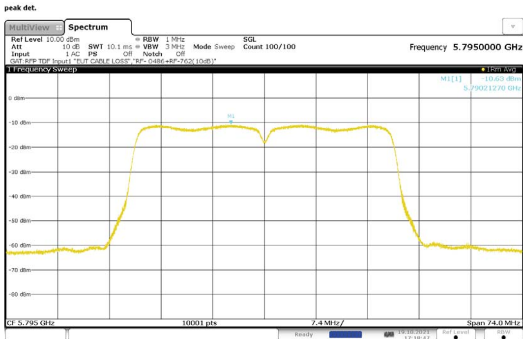
Figure 230: Maximum Power Spectral Density, 802.11n-40, CDD, RF1, 5795MHz
