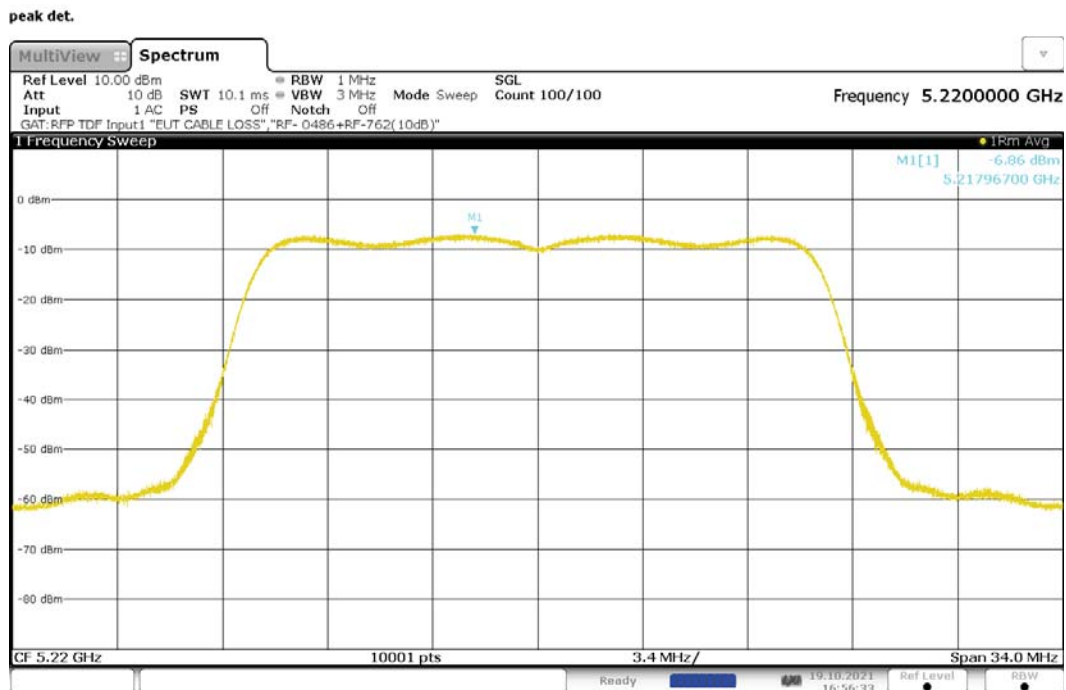
Figure 210: Maximum Power Spectral Density, 802.11ac-20, MIMO, RF1, 5220MHz
