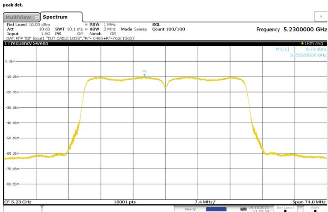
Figure 252: Maximum Power Spectral Density, 802.11ac-40, CDD, RF1, 5230MHz
