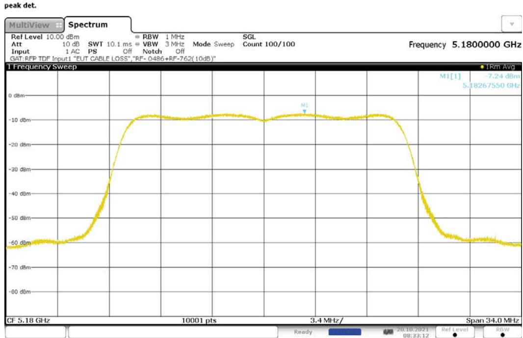
Figure 185: Maximum Power Spectral Density, 802.11ac-20, SISO, RF1, 5180MHz
