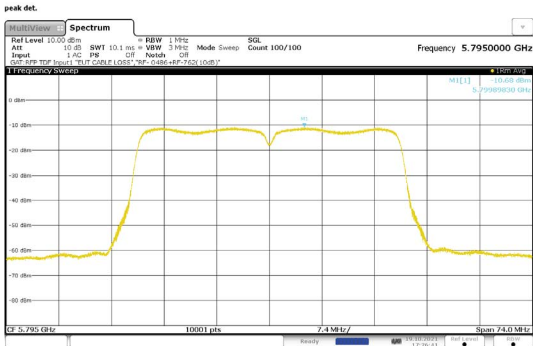
Figure 254: Maximum Power Spectral Density, 802.11ac-40, CDD, RF1, 5795MHz
