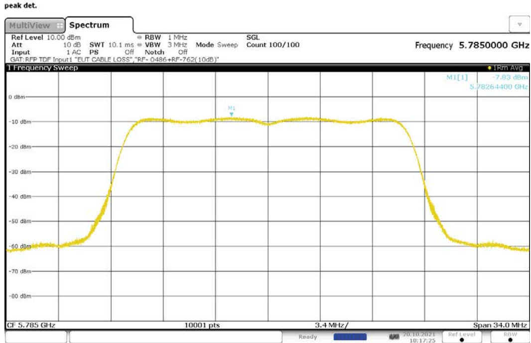
Figure 195: Maximum Power Spectral Density, 802.11ac-20, CDD, RF0, 5785MHz
