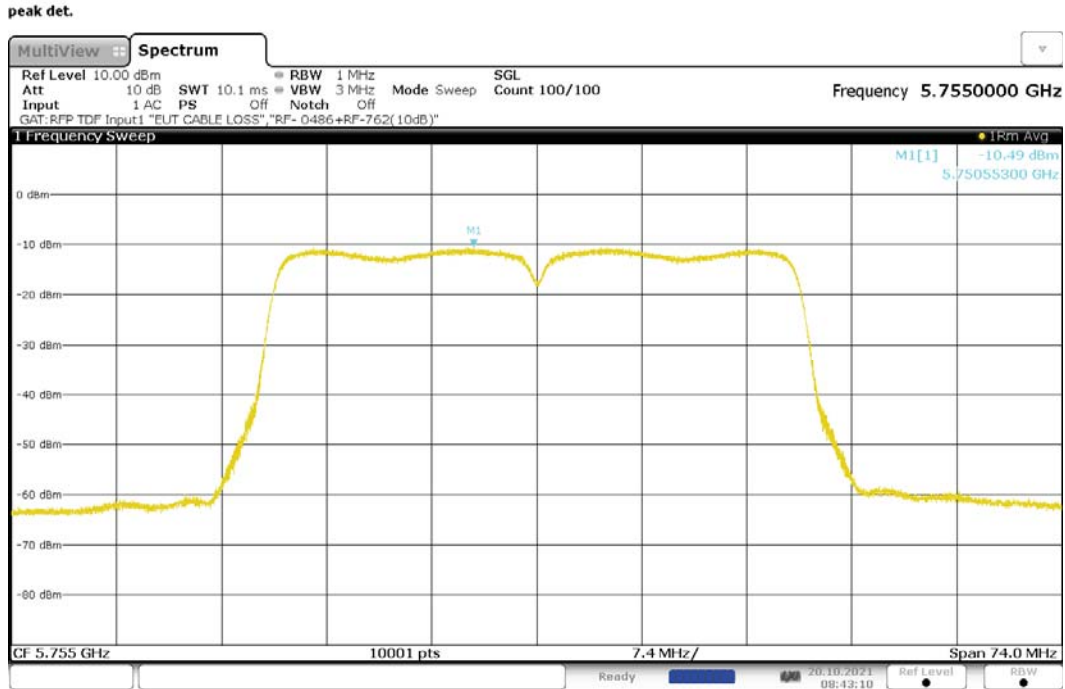
Figure 245: Maximum Power Spectral Density, 802.11ac-40, SISO, RF1, 5755MHz
