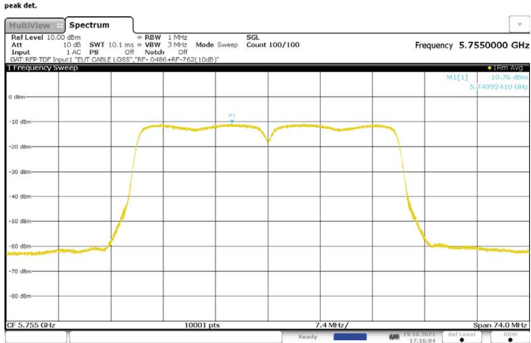
Figure 229: Maximum Power Spectral Density, 802.11n-40, CDD, RF1, 5755MHz
