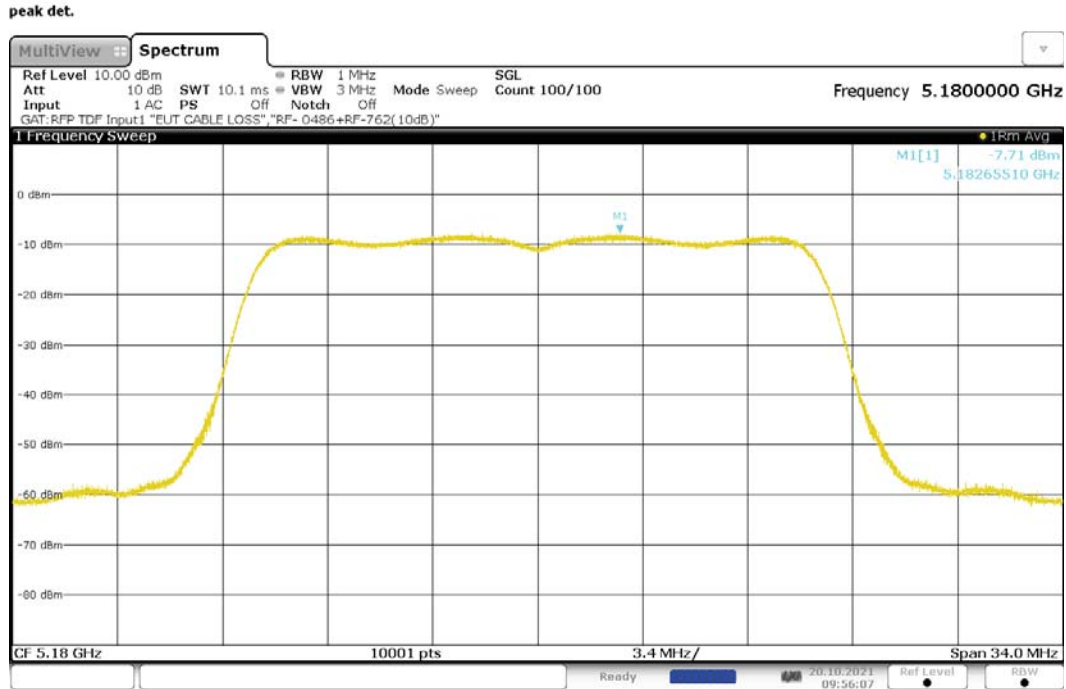
Figure 179: Maximum Power Spectral Density, 802.11ac-20, SISO, RF0, 5180MHz
