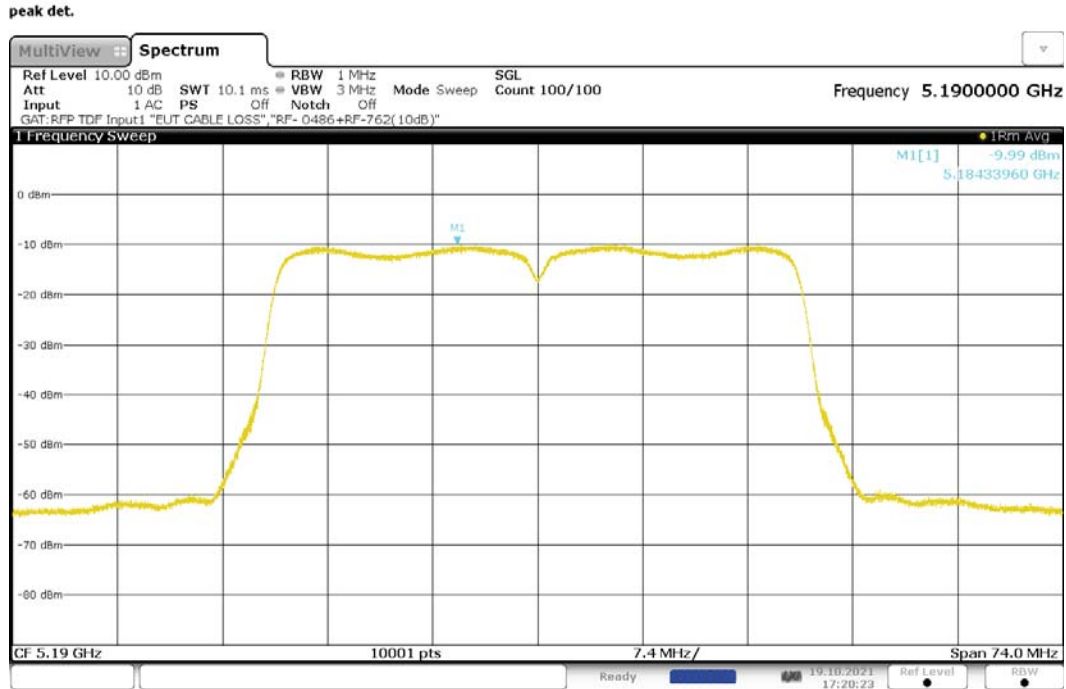
Figure 251: Maximum Power Spectral Density, 802.11ac-40, CDD, RF1, 5190MHz
