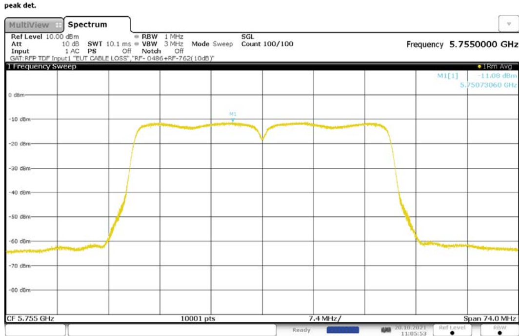
Figure 249: Maximum Power Spectral Density, 802.11ac-40, CDD, RF0, 5755MHz
