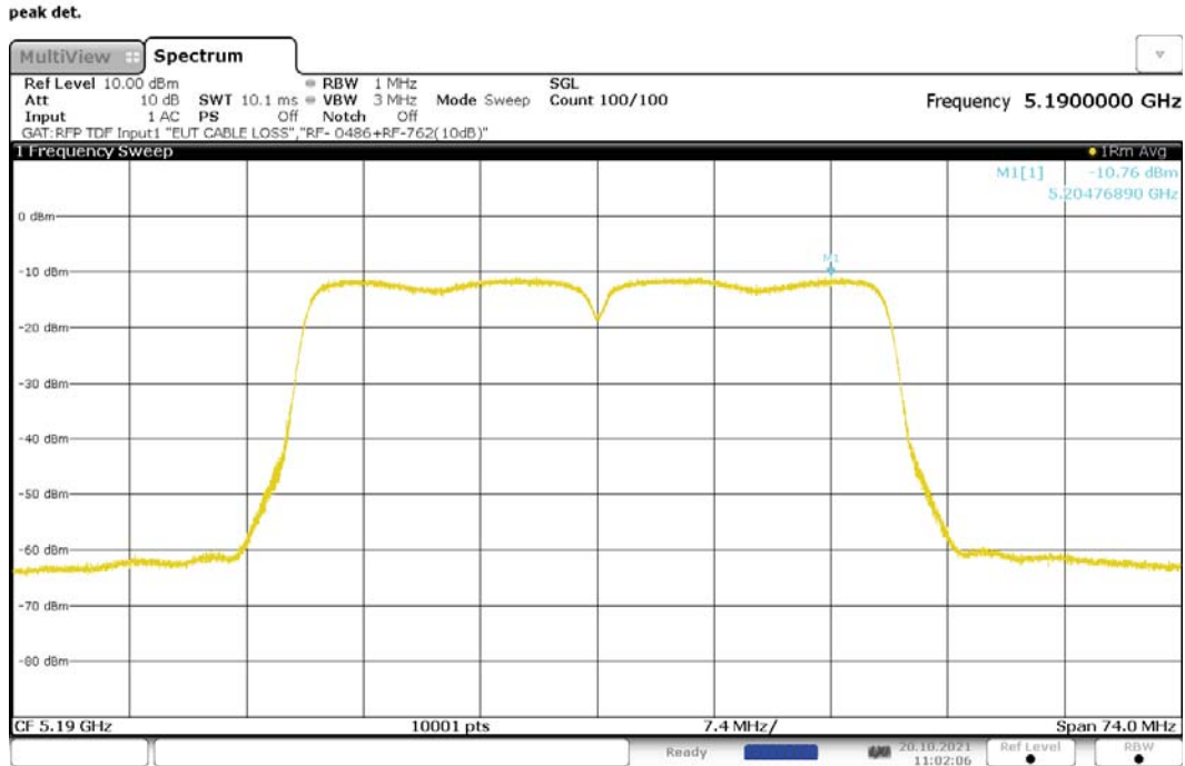
Figure 247: Maximum Power Spectral Density, 802.11ac-40, CDD, RF0, 5190MHz
