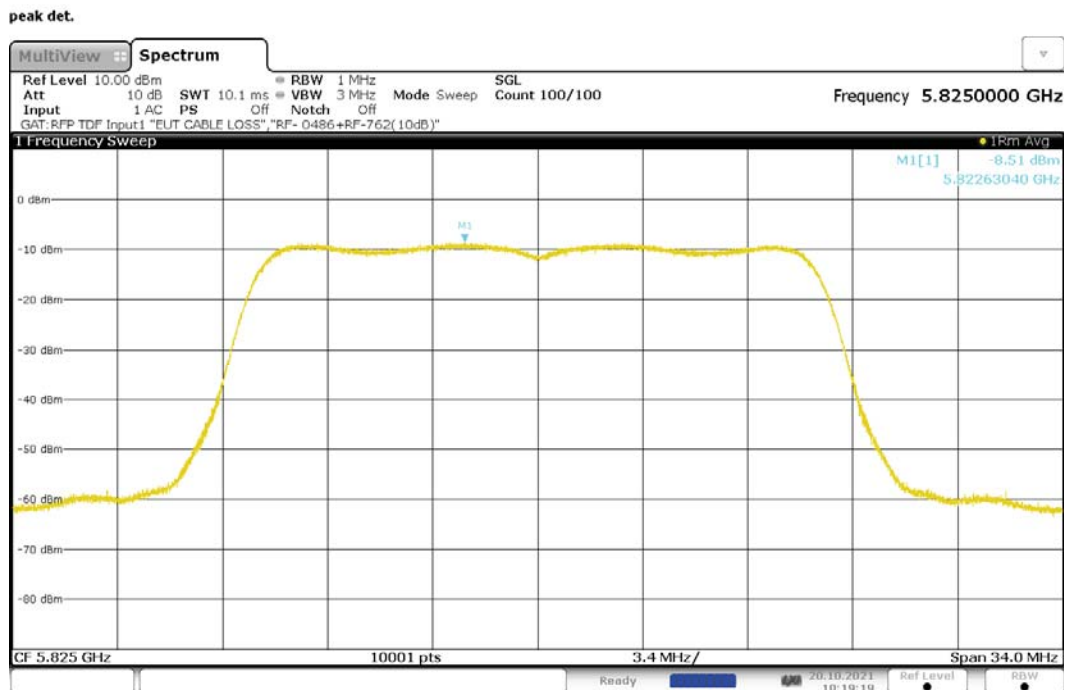
Figure 196: Maximum Power Spectral Density, 802.11ac-20, CDD, RF0, 5825MHz
