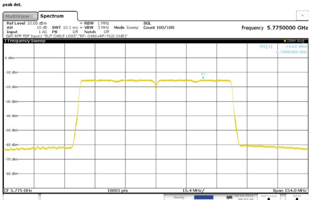
Figure 264: Maximum Power Spectral Density, 802.11ac-80, SISO, RF0, 5775MHz
