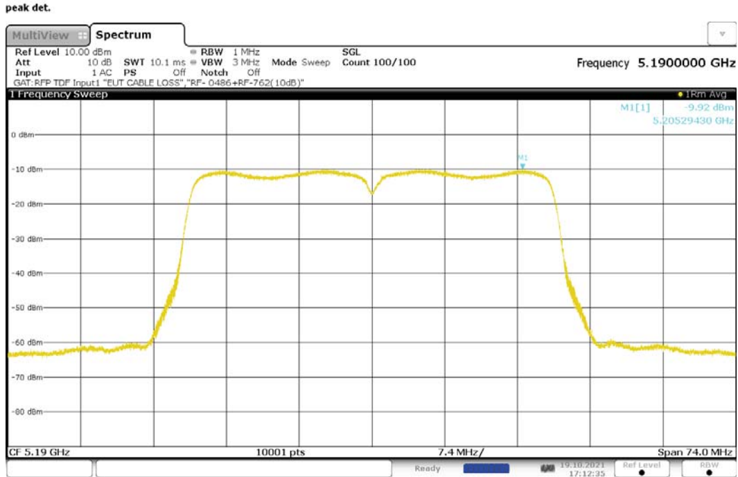
Figure 231: Maximum Power Spectral Density, 802.11n-40, MIMO, RF0, 5190MHz
