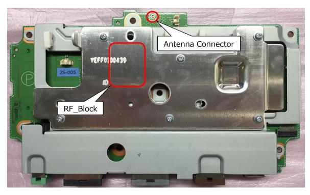
Fig.4 WLAN\_PCB (w/ Heat Sink) [Surface-Side]
