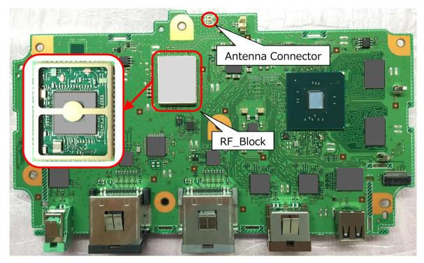
Fig.5 WLAN\_PCB (w/o Heat Sink) [Surface-Side]
