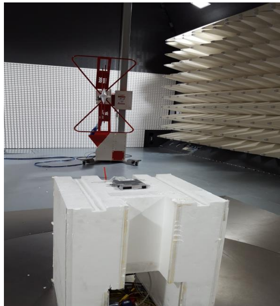
Figure C6. DUT Setup - Radiated
