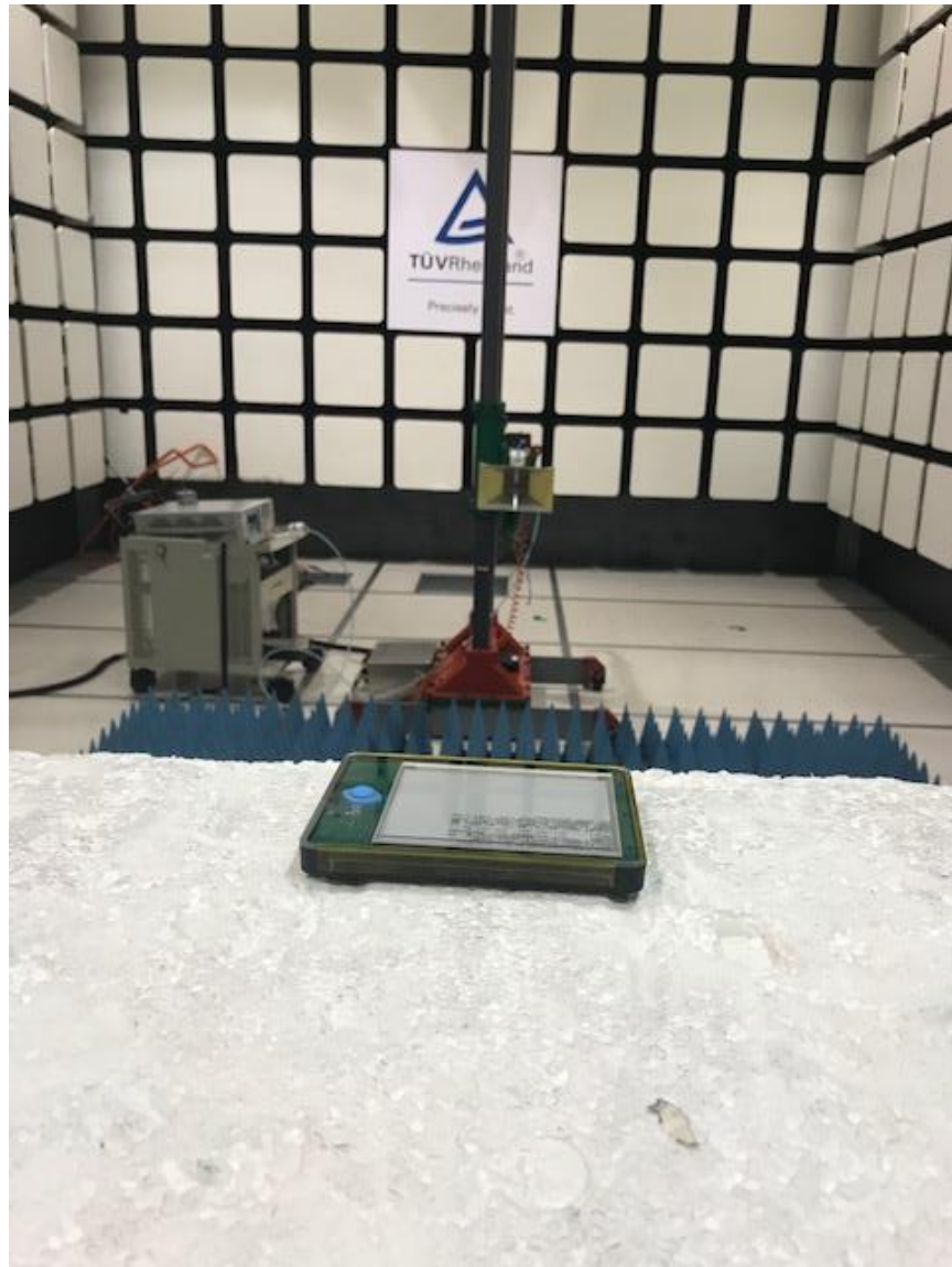
Figure 31: 1 GHz – 6GHz Radiated Emission Test Setup – Rear View
