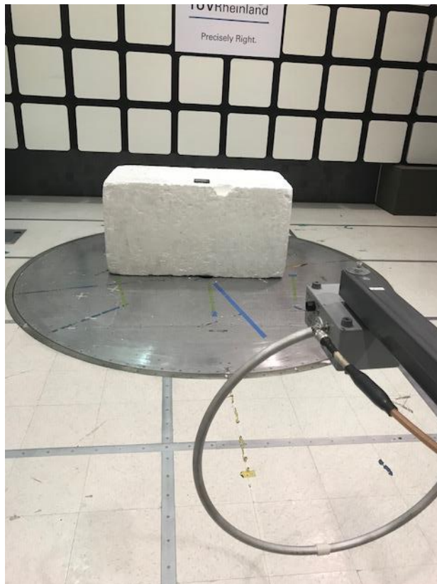
Figure 26: 9 – 30,000 kHz Radiated Emission Test Setup – Rear View
