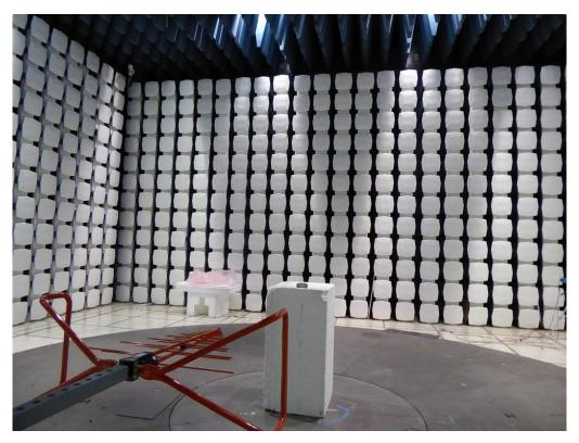
Figure 28: 30 - 1000 MHz Radiated Emission Test Setup – Rear View
