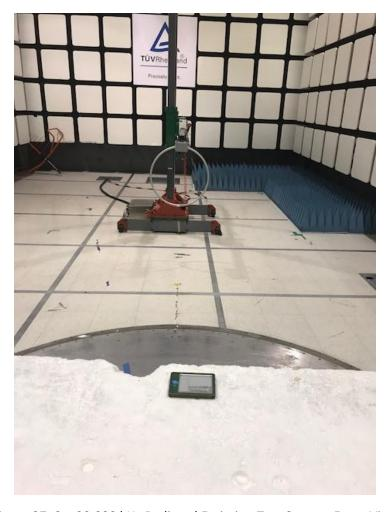
Figure 27: 9 – 30,000 kHz Radiated Emission Test Setup – Front View
