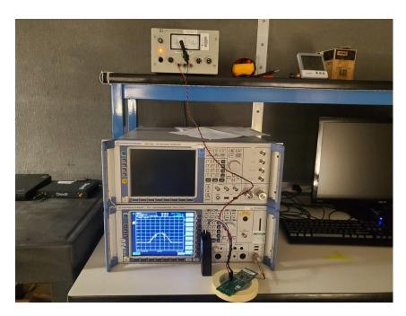
Figure 25: Photo of Conducted Tabletop Setup
