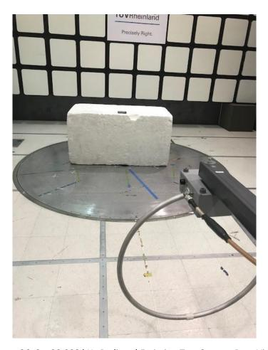
Figure 26: 9 - 30,000 kHz Radiated Emission Test Setup – Rear View
