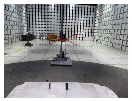
Figure 29: 30 - 1000 MHz Radiated Emission Test Setup – Front View
