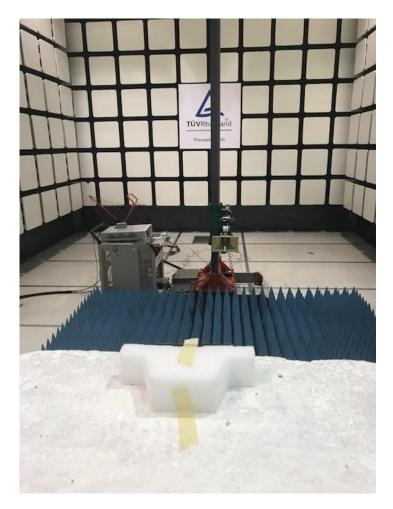
Figure 31: 1 GHz – 6GHz Radiated Emission Test Setup – Rear View
