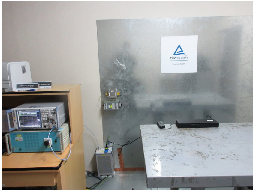
Photograph 7: Set-up for AC Mains (Front View)
