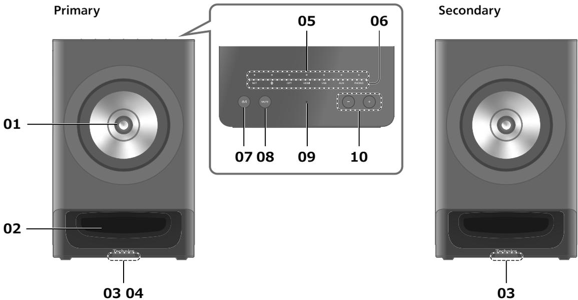
**01 Speaker unit (Coaxial 2-way unit)****02 Bass reflex port****03 Power indicator**
